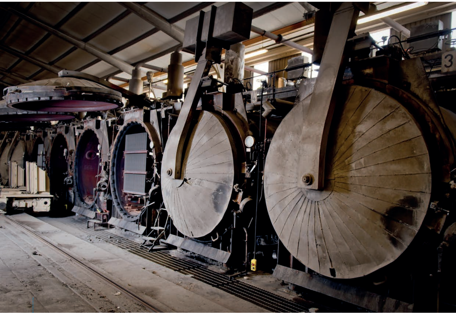
The giant autoclaves in which the aircrete blocks are cured.
