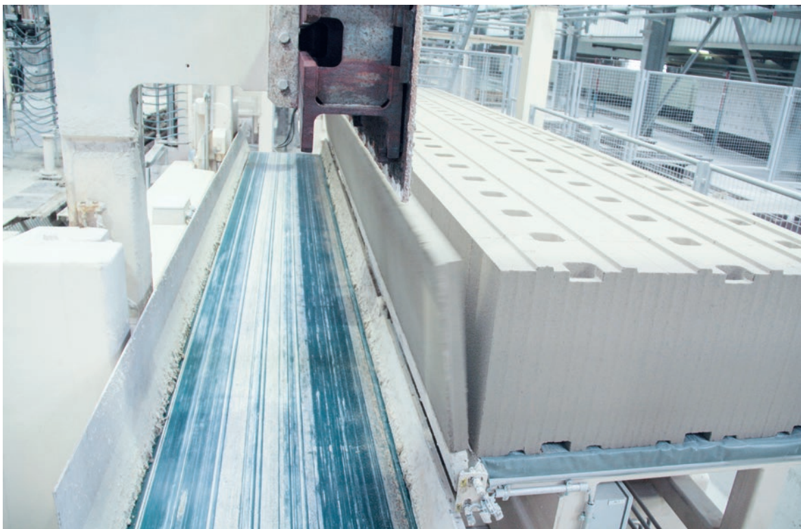
Fig. 3: The Wehrhahn bed remover removes the bottom layer before autoclaving, allowing the fresh material to be recycled through the returns slurry system.
