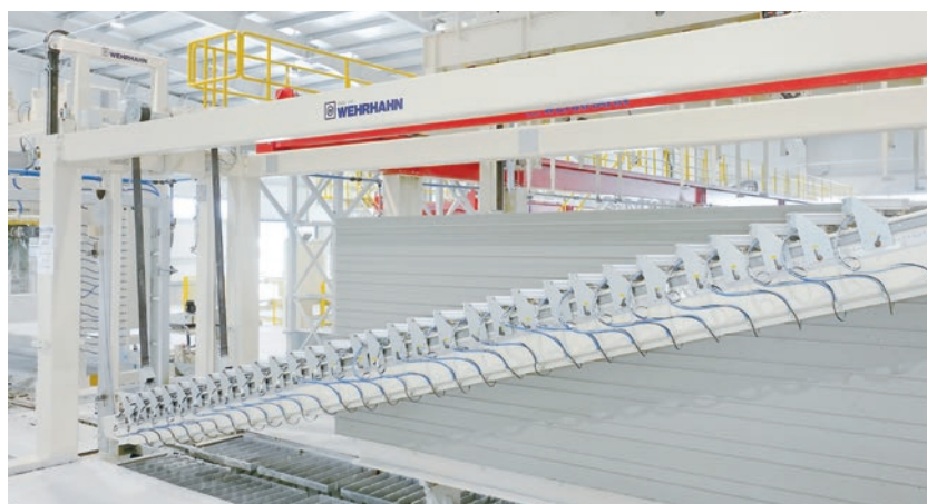
Fig. 1: The redesigned Smart thickness cutter uses longitudinally staggered cutting wires to reduce local loading on the green cake, particularly when producing 50 mm and 75 mm products.
