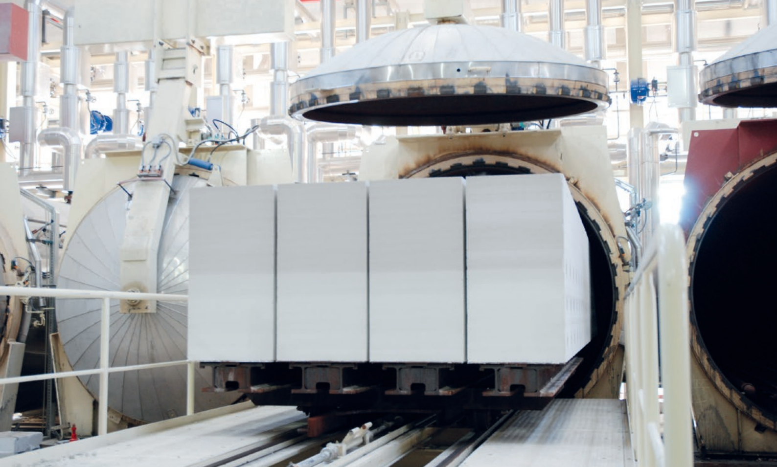
Fig. 2: Upright cakes on an autoclave trolley in the Plus process. The horizontal thickness-cutting joints are separated after autoclaving.
