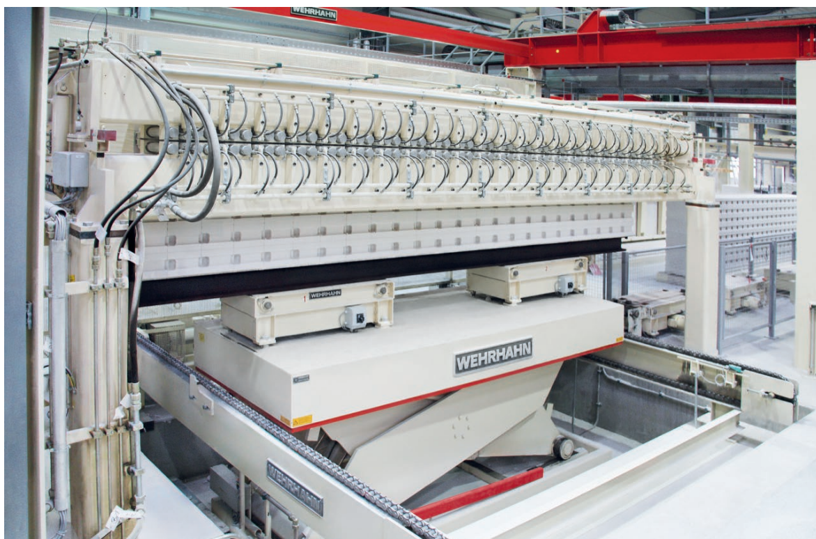
Fig. 4: The Wehrhahn white separator opens the thickness-cutting joints in the hardened cake, with machine settings adapted to product density and thickness.
