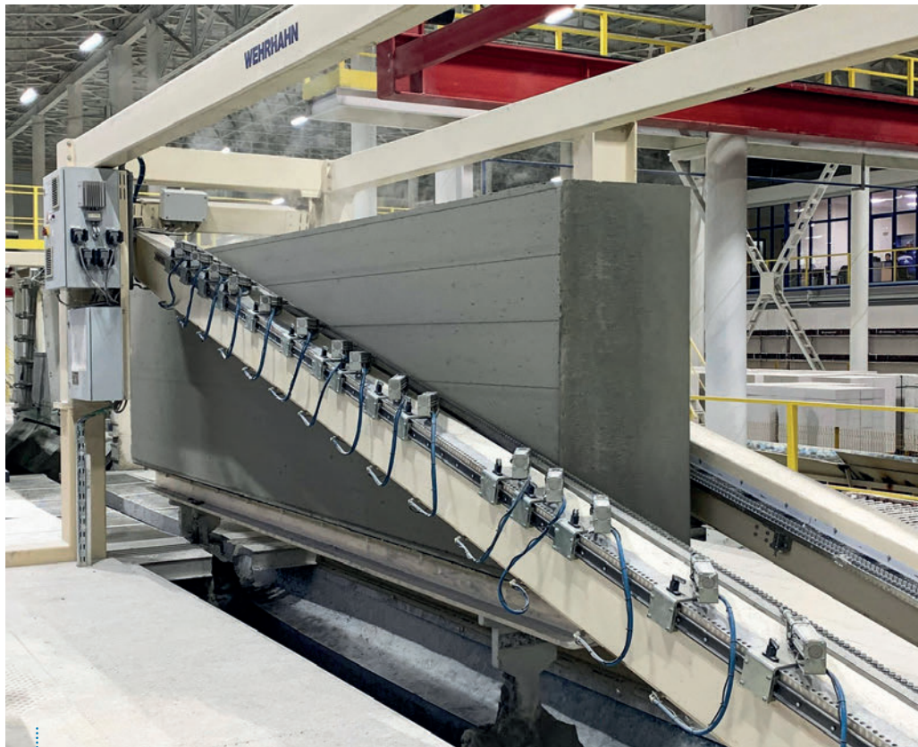
Fig. 3: Uniform distribution of cutting wires reduces stress during thickness cutting
