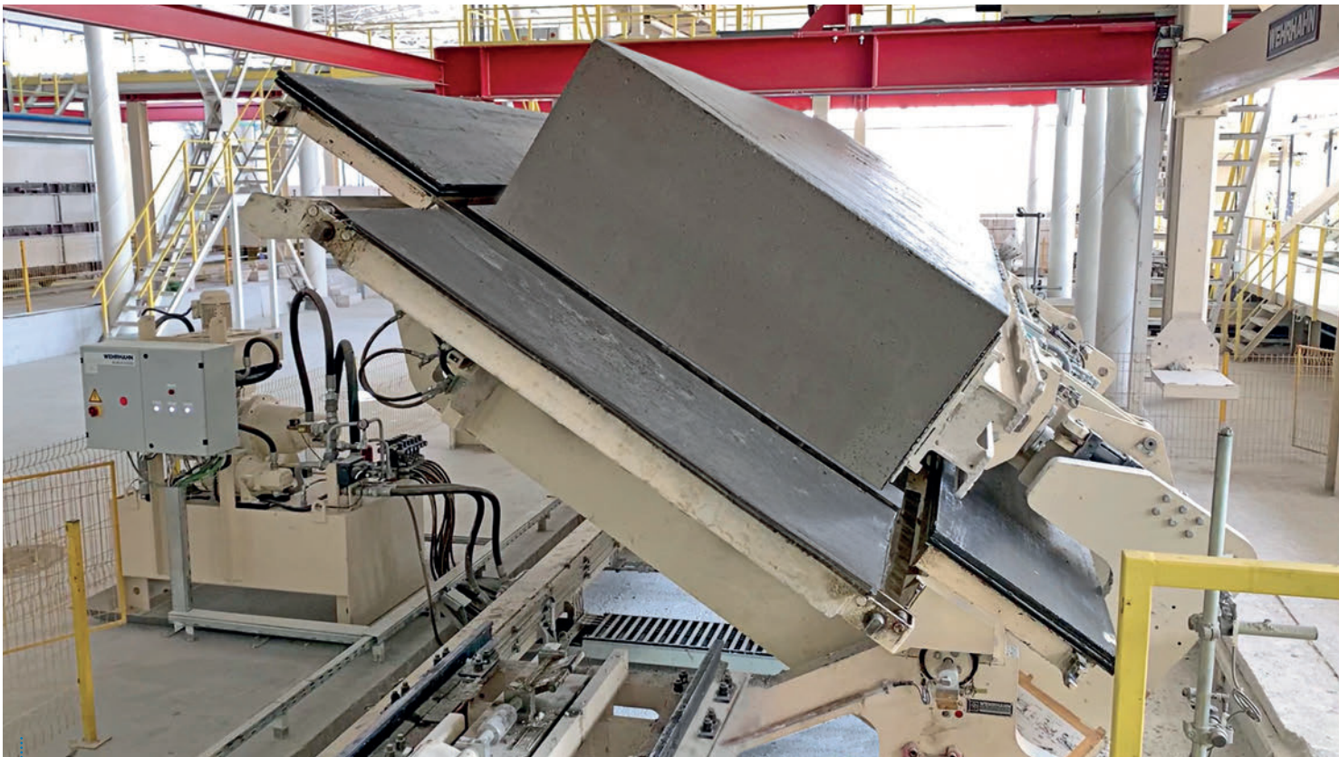
Fig. 1: Tilt cutting: less binders and shorter precuring times
