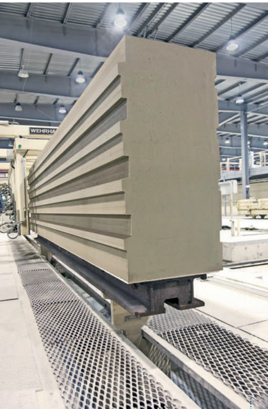
Fig. 2: Easy and precise profiling in tilt cutting systems
