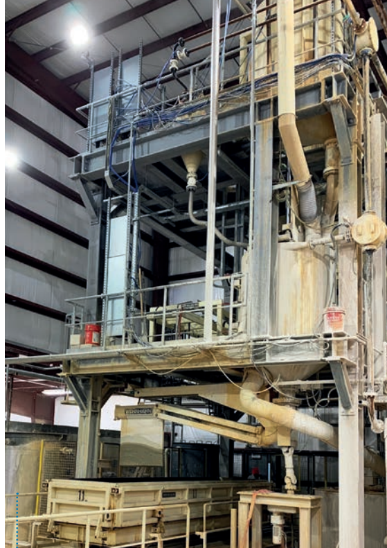
The mixing unit combines a large number of equipment and is controlled by a single system: Wecomix.
