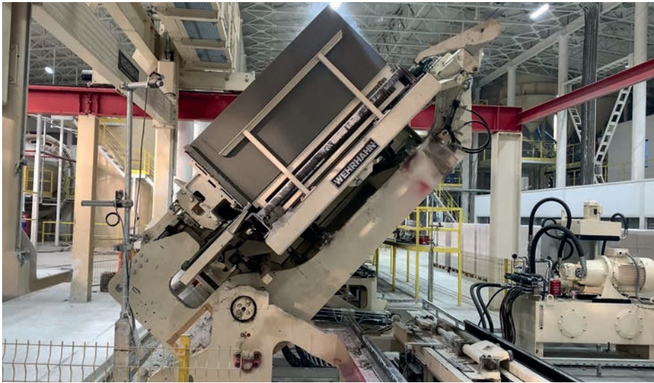
The universal tilting machine is set on floor level, tilting the flat cake for cutting and tilting it back for autoclaving.
