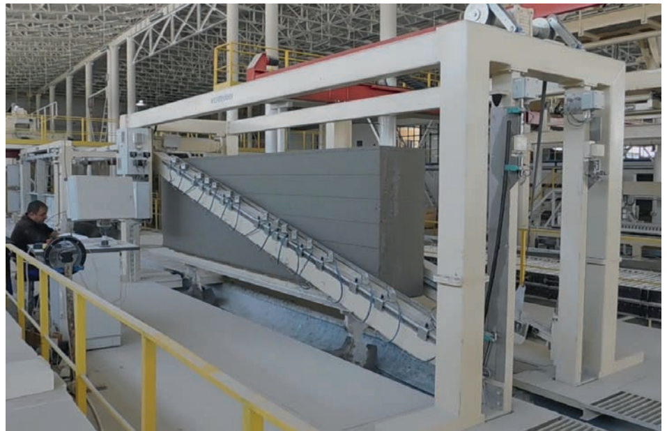
Cutting line with latest high precision thickness cutter.
