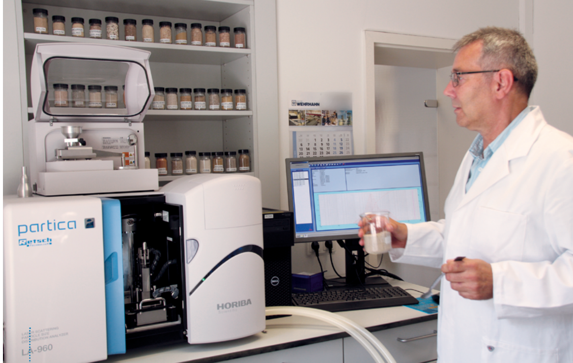
A laser scattering particle size distribution analyser even detects particles down to 0.1 \mu\text{m} in detail, whereas traditional sieving methods with air jet sieving or vibration screening machines are limited to 32 \mu\text{m} .
