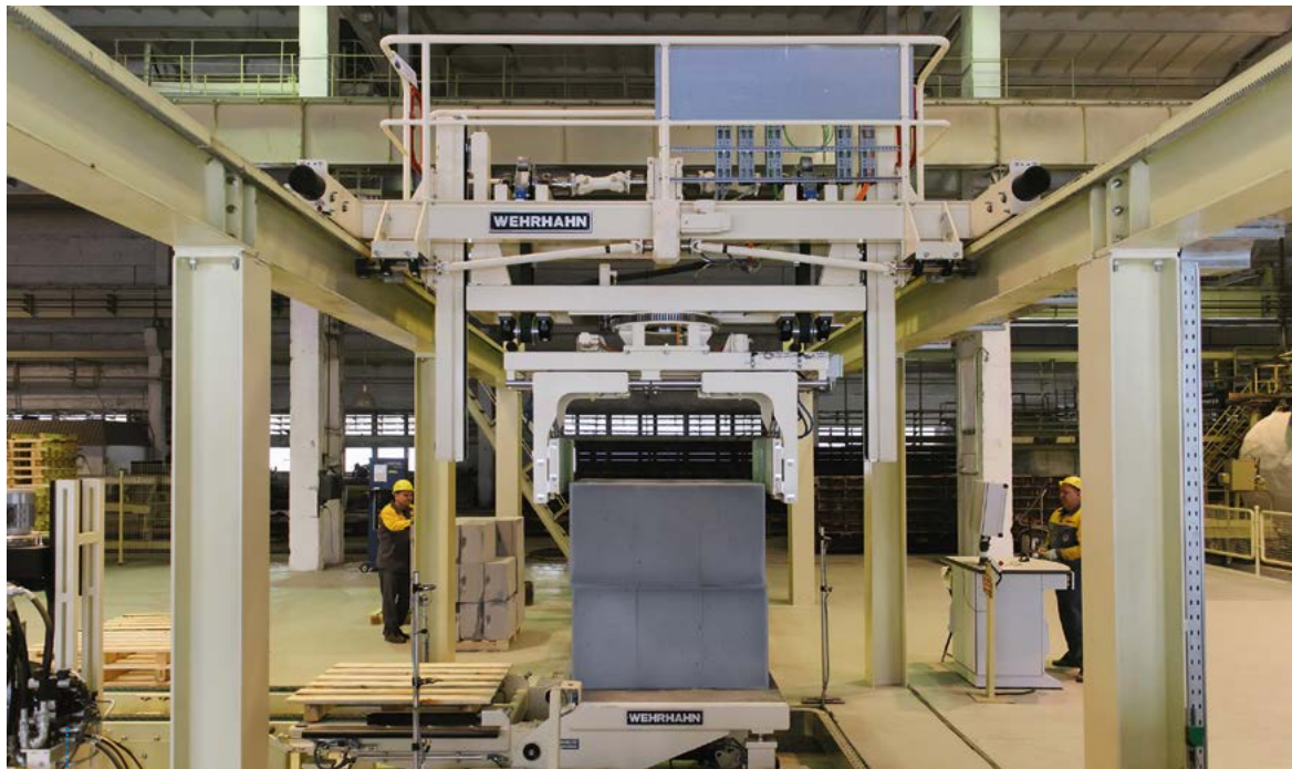
The new sorting and packing line is equipped with the highly efficient Wehrhahn pack maker, tilting table and stacker for sorting and making packs up to 1.8 m height. Blocks with tongue and groove can also be handled.
