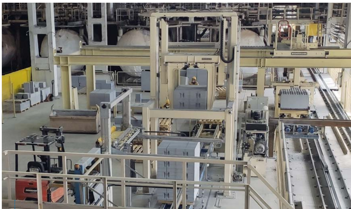
Modernisation stage 1 and 3: the new sorting and packing line allows sorting, tilting, turning, stacking, shrink-wrapping and strapping of packs even for long distance transportation.
