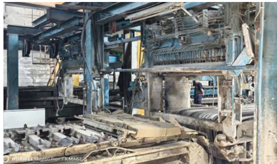
Old inefficient horizontal cake cutting system
