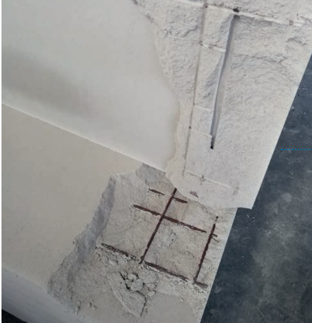
Fig. 4: Typical crack pattern occurring after a faulty autoclaving process.
