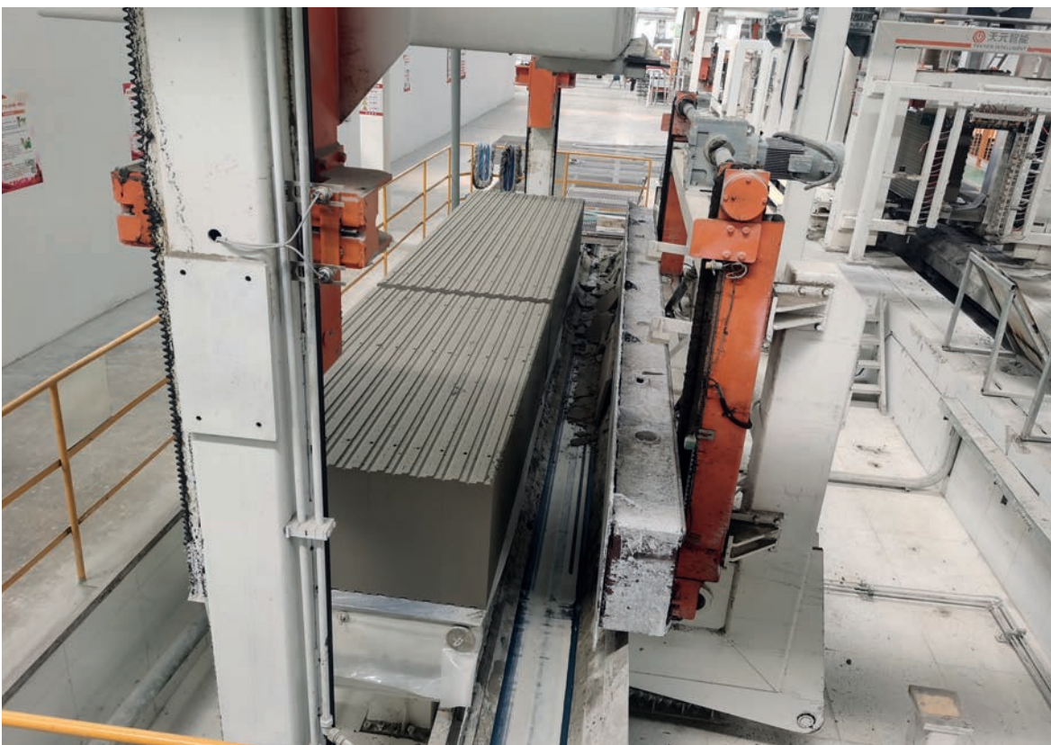
Dry material conveying device under the tilting table.
