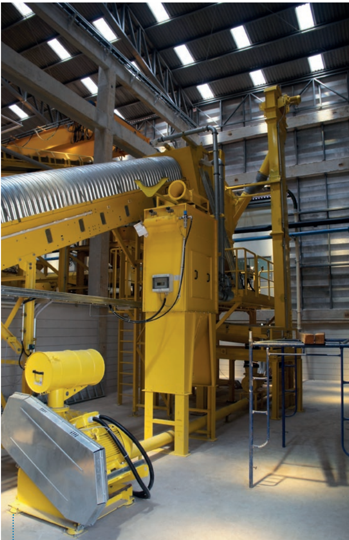
Crushing plant for fine crushing of the material (level 2) and transport to an intermediate silo.
