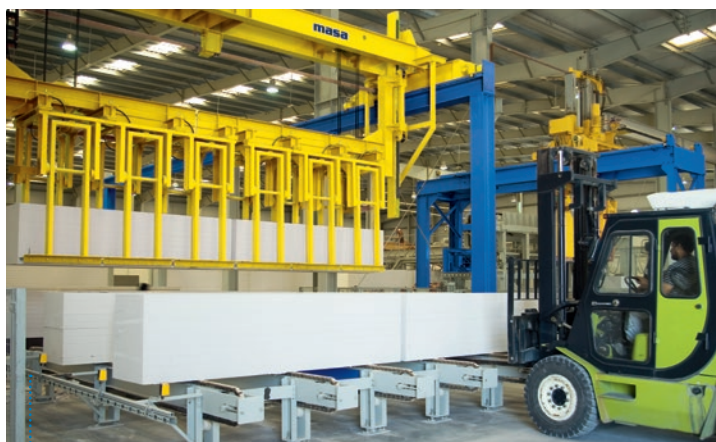
The block transfer device of the Vario Block line passes the reinforced products to the separate packaging line.
