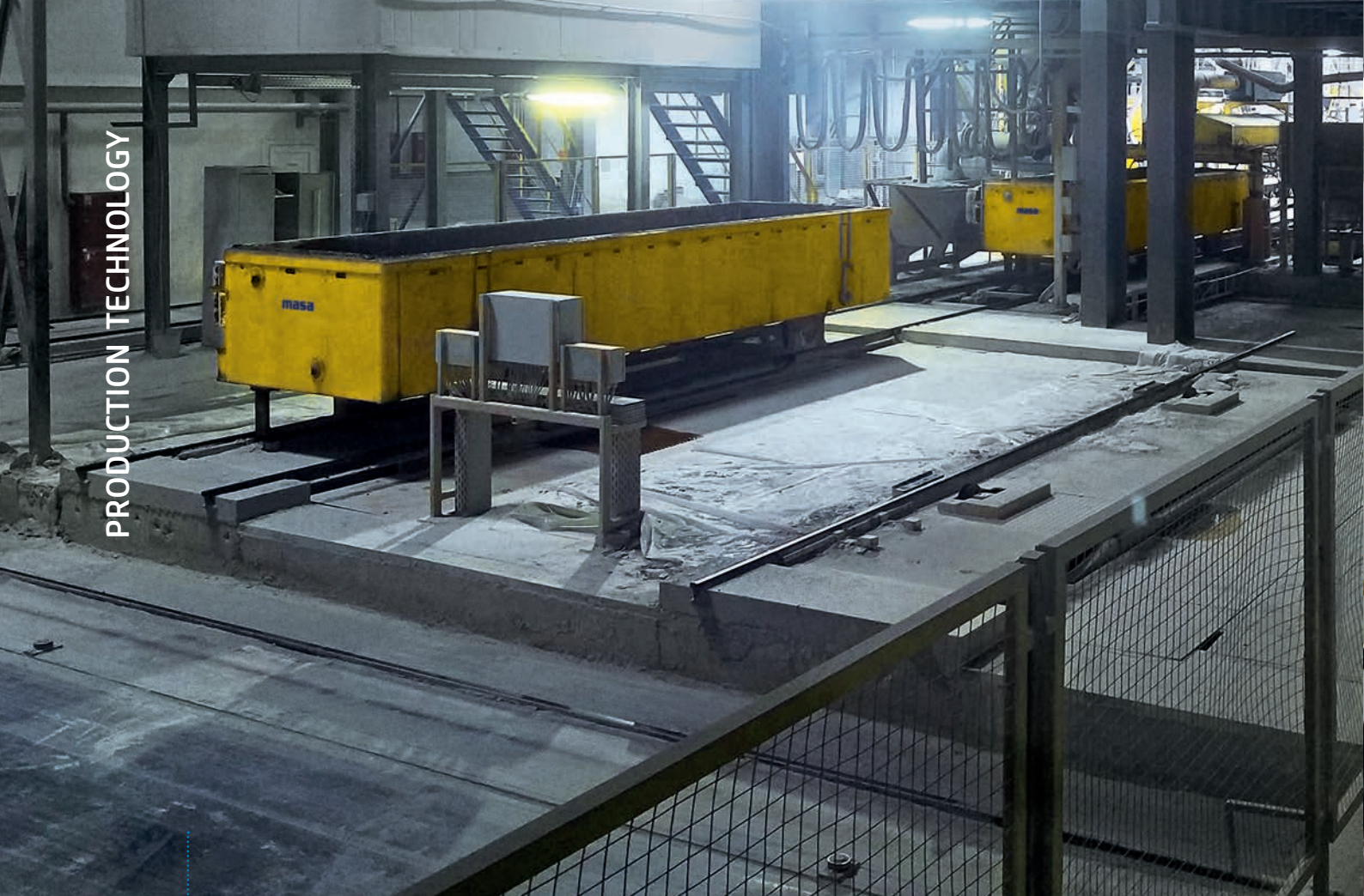
Fig. 3: After the filling process the filled mould is moved to the bouncing table
