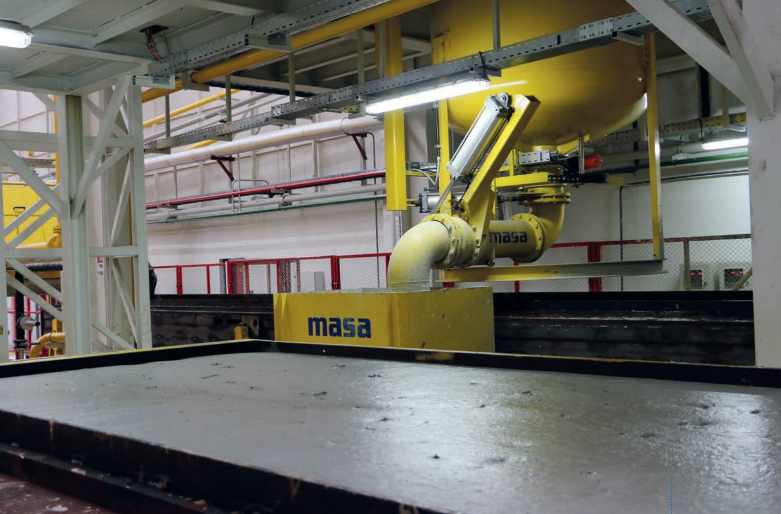
Fig. 4: When the mixing process has been completed, the casting device feeds the mixture into a casting mould.
