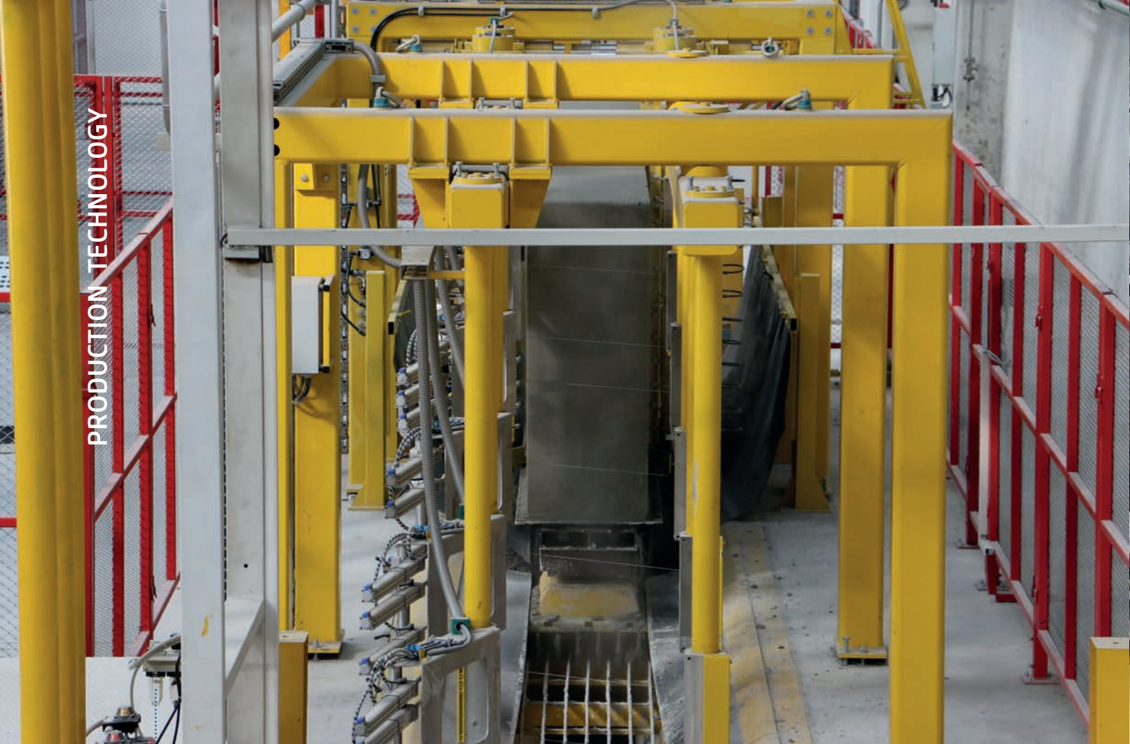
Fig. 5: Cutting line: As the aerated concrete block stands upright, it is possible to use short cutting wires. These enable highly precise geometrical cuts.
