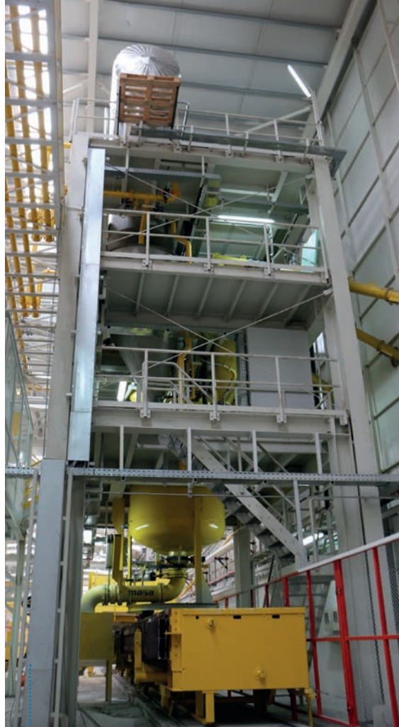
Fig. 2: Dosing, mixing, casting: The complete mixing tower with its different levels is characterized by its compact design.
