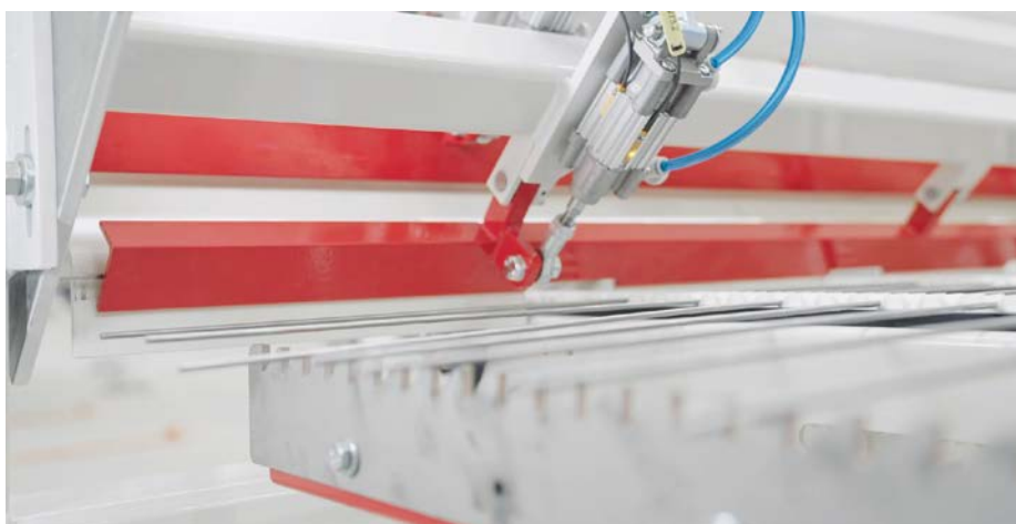
Placing of the wires on the positioning unit.
