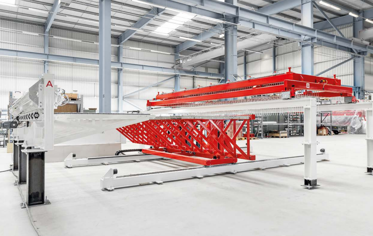
Wire Handling System: Smart technology for automated positioning of reinforcement wires.
