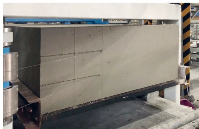
Lintel Cutter producing lintels with a height of 200 mm.
