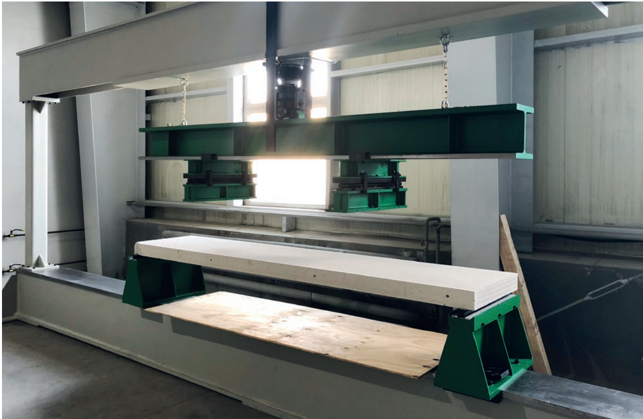
Flexible test equipment for products with a length up to six metres.
