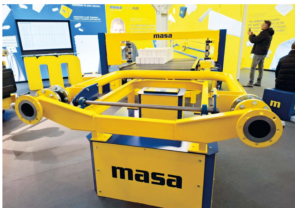
Pipe Loop Scale for automatic calculation of slurry density.
