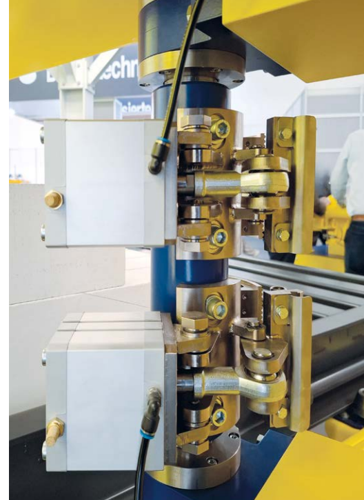
The cutting wires are tensioned pneumatically in the wire unit.
