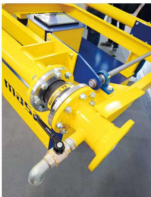
Compensator, outlet for sampling and weighing device.
