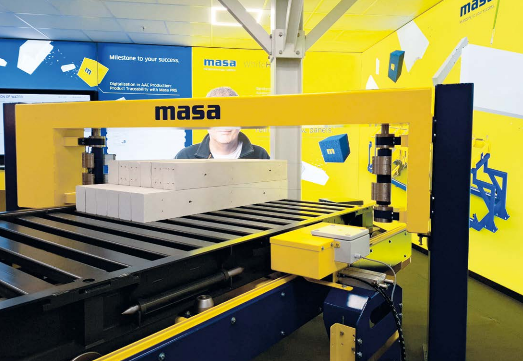
The linter cutter is an ideal addition to the cutting plant.
