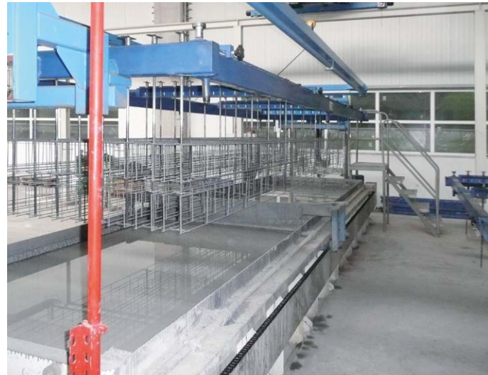
Step 1: The reinforcement is protected against corrosion by immersion in a coating bath.
