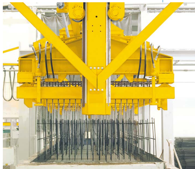
Step 3: The entire reinforcement is inserted into the fresh cake.
