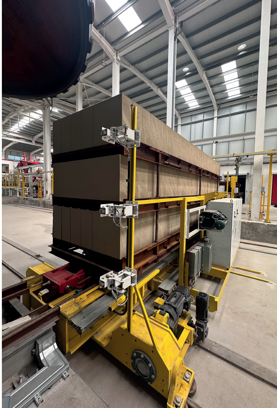
Cakes on tagged hardening grids on the way to hardening.
