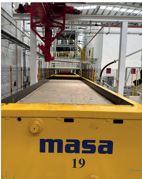
Mould and mould side part: RFID tagging.
