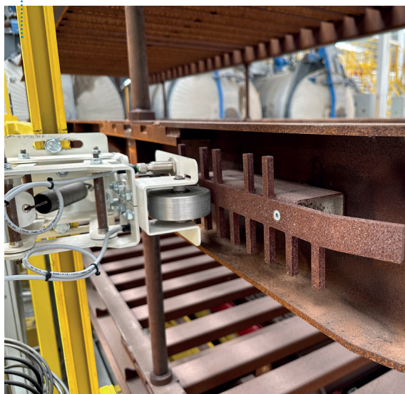
Reader for binary coding on the hardening grid.
