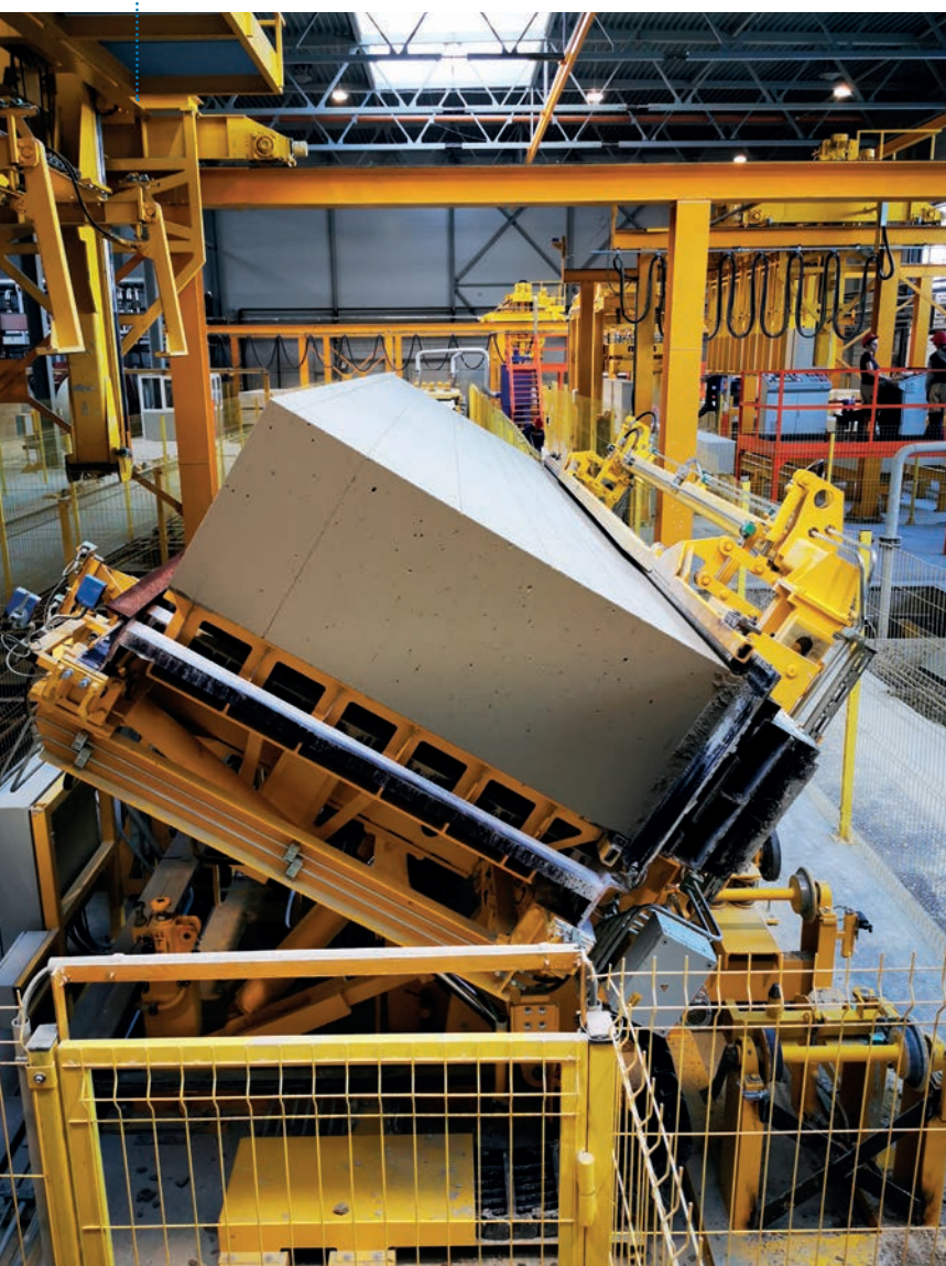
Tilting table behind the cutting plant for flat stacking of the products inside the autoclaves
