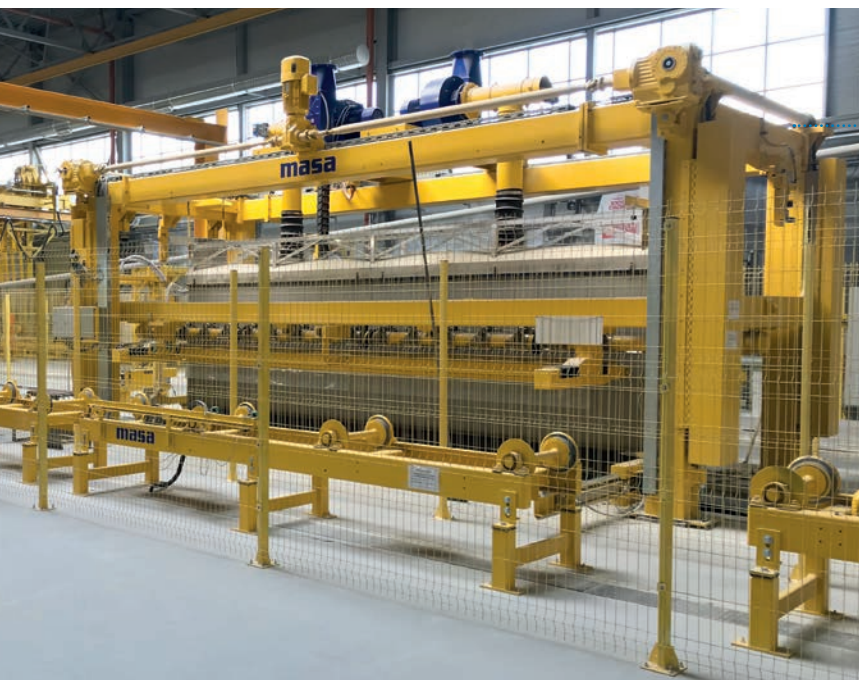
Tilting table behind the cutting plant for flat stacking of the products inside the autoclaves
