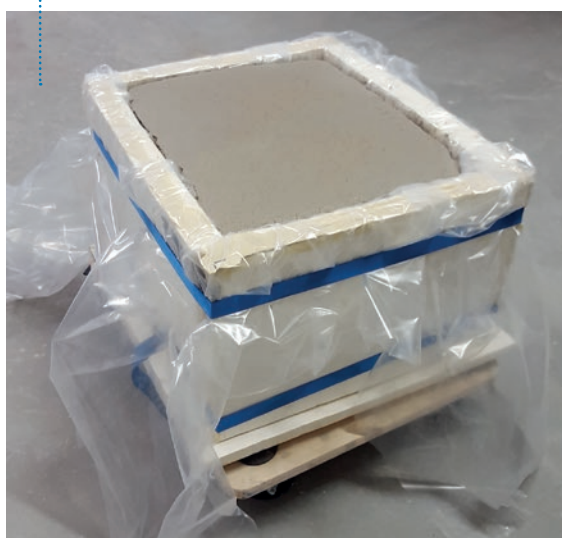
Casting mold for sample blocks
