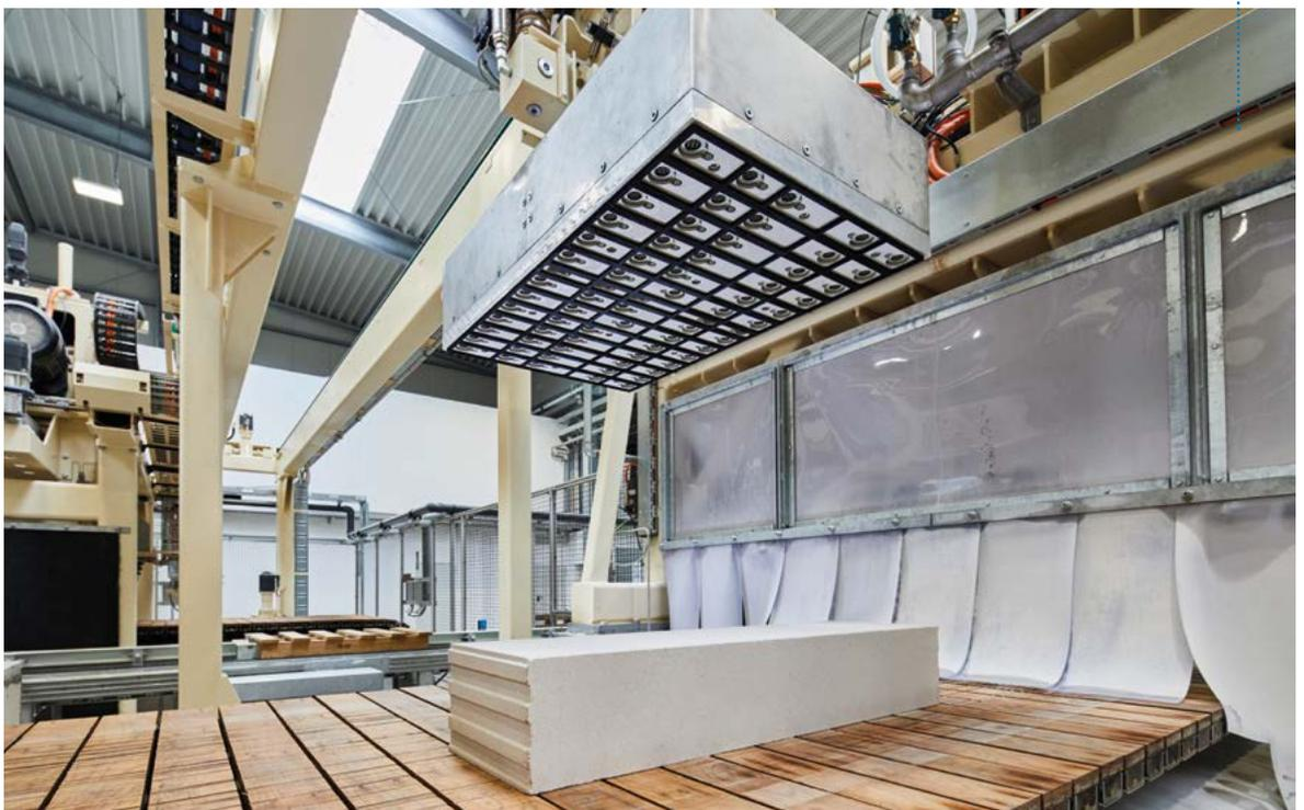
*The finished products are placed on wooden pallets, secured for transport, and labelled with an automatic labelling device.*
