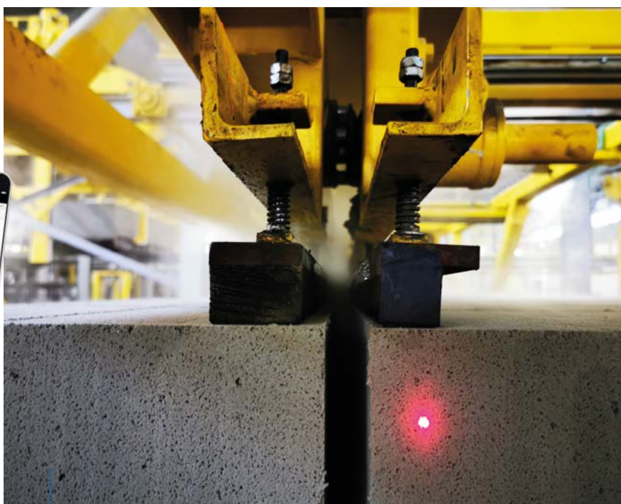
Use of the latest measurement technology for exact positioning of the cakes and control of the movements
