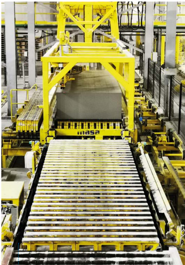
Aerated concrete cake in the green separating table
