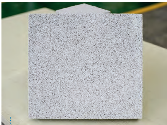
Heyue AAC block incorporating ceramic polishing powder
