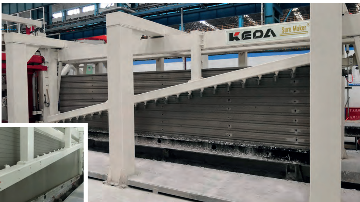
Cable-stayed beam horizontal cutting machine
