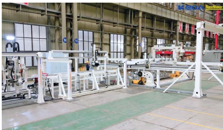
K-ARFAS, the Automatic Reinforcement Cage Assembly System developed by Keda Suremaker.
