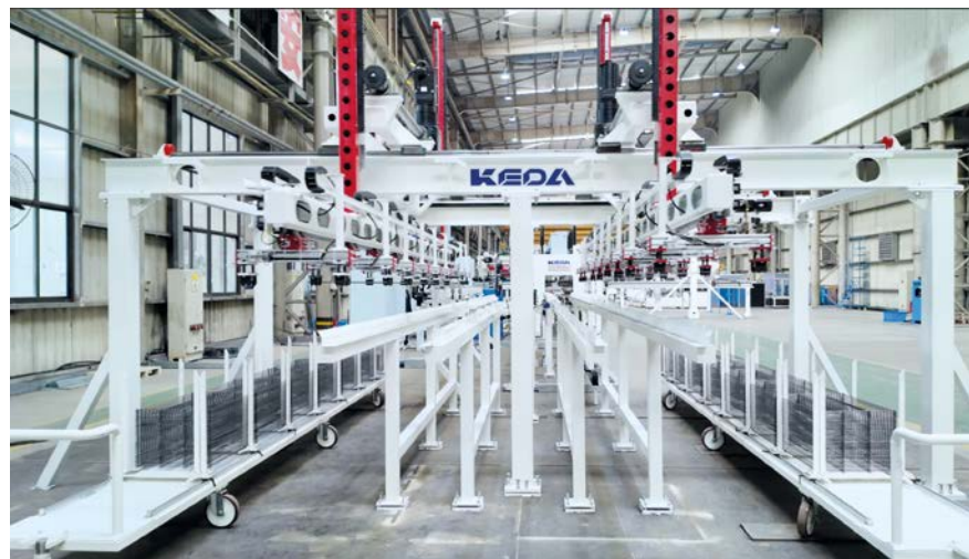
Automatic mesh panel gripping and reinforcement cage welding.
