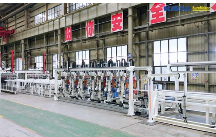
K-ARFAS, the Automatic Reinforcement Cage Assembly System developed by Keda Suremaker.
