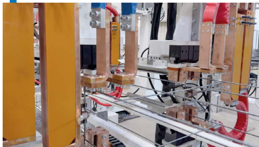
Automatic mesh panel gripping and reinforcement cage welding.
