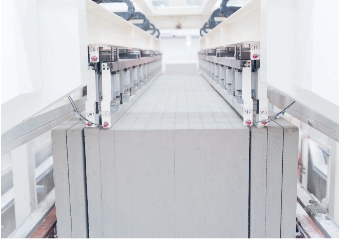
Intelligent Dual-Sided Green Cake Separation – the dual-sided grippers synchronize their actions to split the entire green body in one go.
