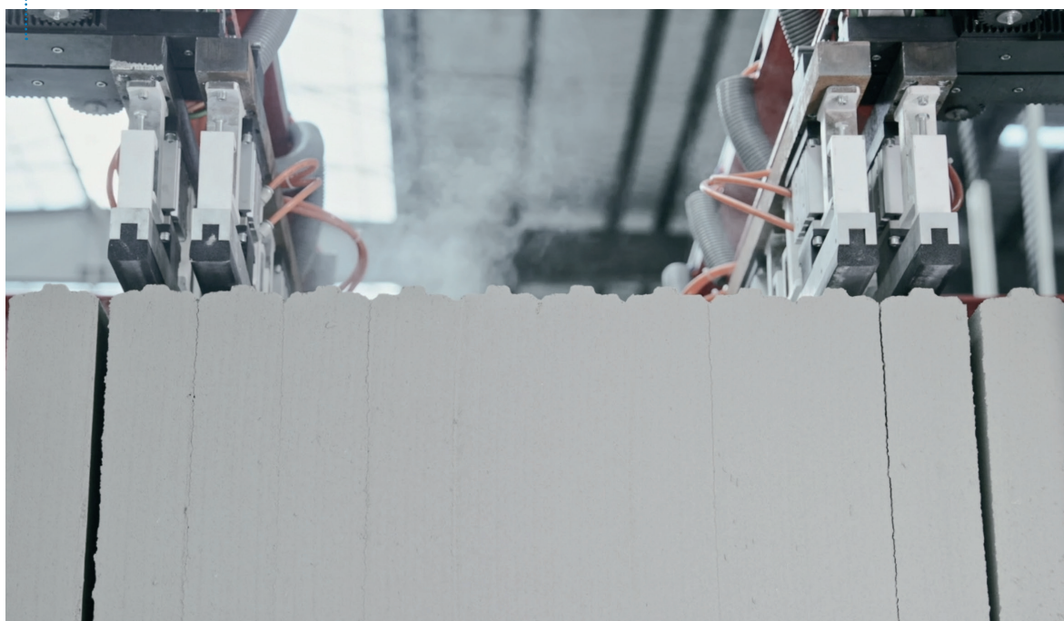
Fig. 6: Intelligent dual-sided synchronous separation improves production efficiency.
