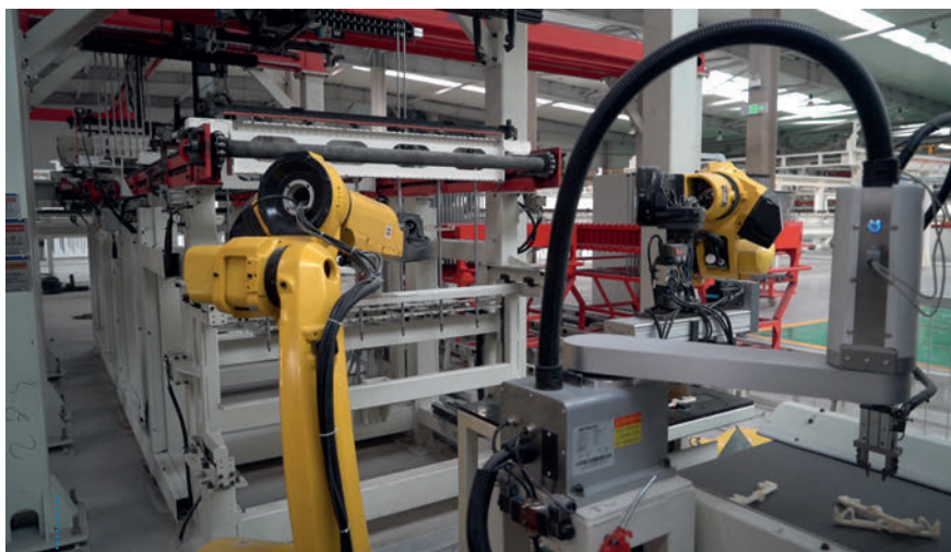
Intelligent steel reinforcement cage meshing cage technology in the BBMG Shanxi Plant.
