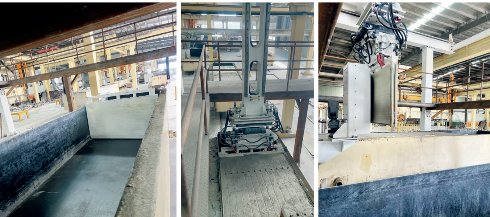
Strict control of raw material waste: Precise partition positioning and synchronous control effectively avoid issues like slurry overflow and moulding deviations.
