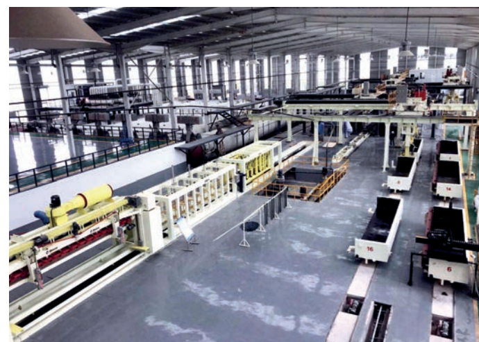
Shandong Zhongchang Development and Construction Group Co., Ltd. is using gold mine tailings in AAC production.
