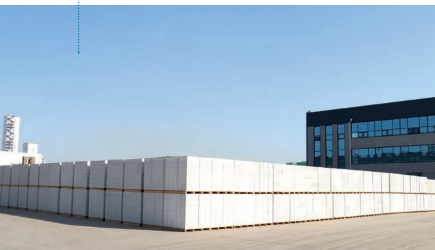
Shandong Zhongchang Development and Construction Group Co., Ltd. is using gold mine tailings in AAC production.
