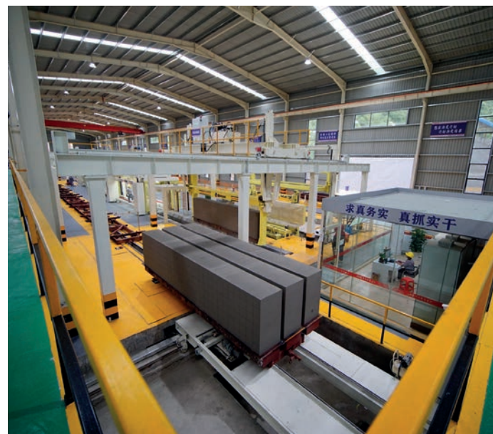
Granite saw mud is used in the Hezhou Huada New Building Materials Co., Ltd. production facility.
