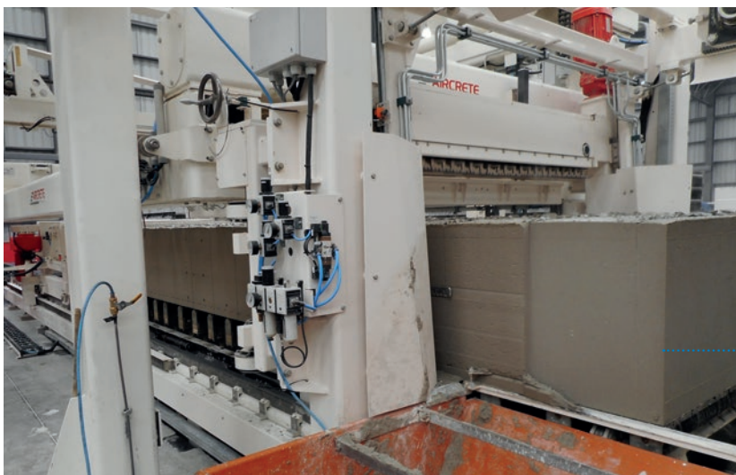
Fig. 8: High-Speed Cutting Frame with double wire cut for Super Smooth surfaces
