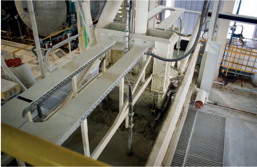
Fig. 12: A homogeneous mix and the filling of the mould is the key to achieving a good AAC cake
