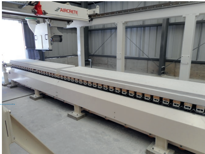
Fig. 13: Aircrete AAC panel milling and sawing line
