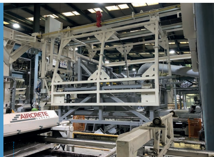
Fig. 3: The vacuum crane is repositioned and attached to a new vacuum hood crane for efficient top waste collection.
