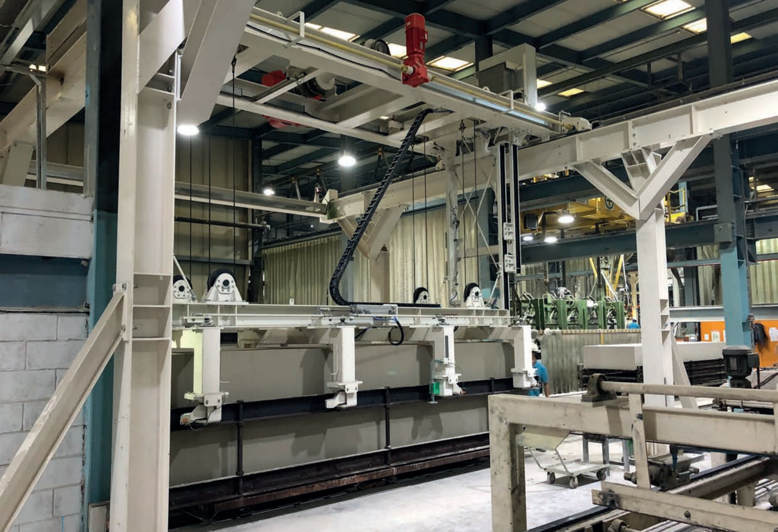
Fig. 4: The new frame stacking crane picks the cake automatically and stacks it two or three high as per the autoclave height.
