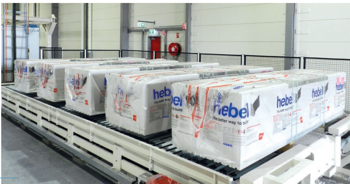
Fig. 7: Ready AAC panels buffering on the line while at the back AAC walls provide structure to the hall.
