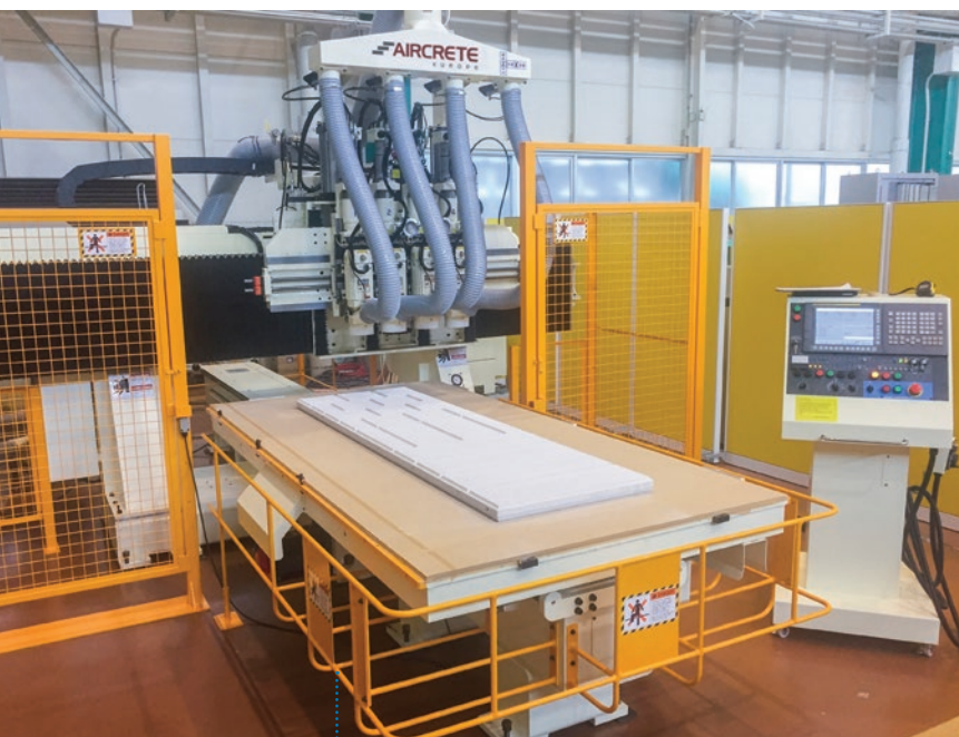
Fig. 8: Aircrete panel milling system.
