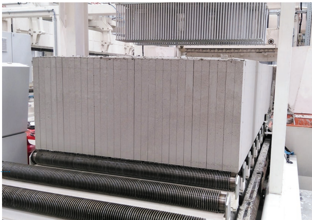
Fig. 4: Flat-cake cutting enables all the cuts on the cake remain open after cutting, ensuring no risks of sticking.
