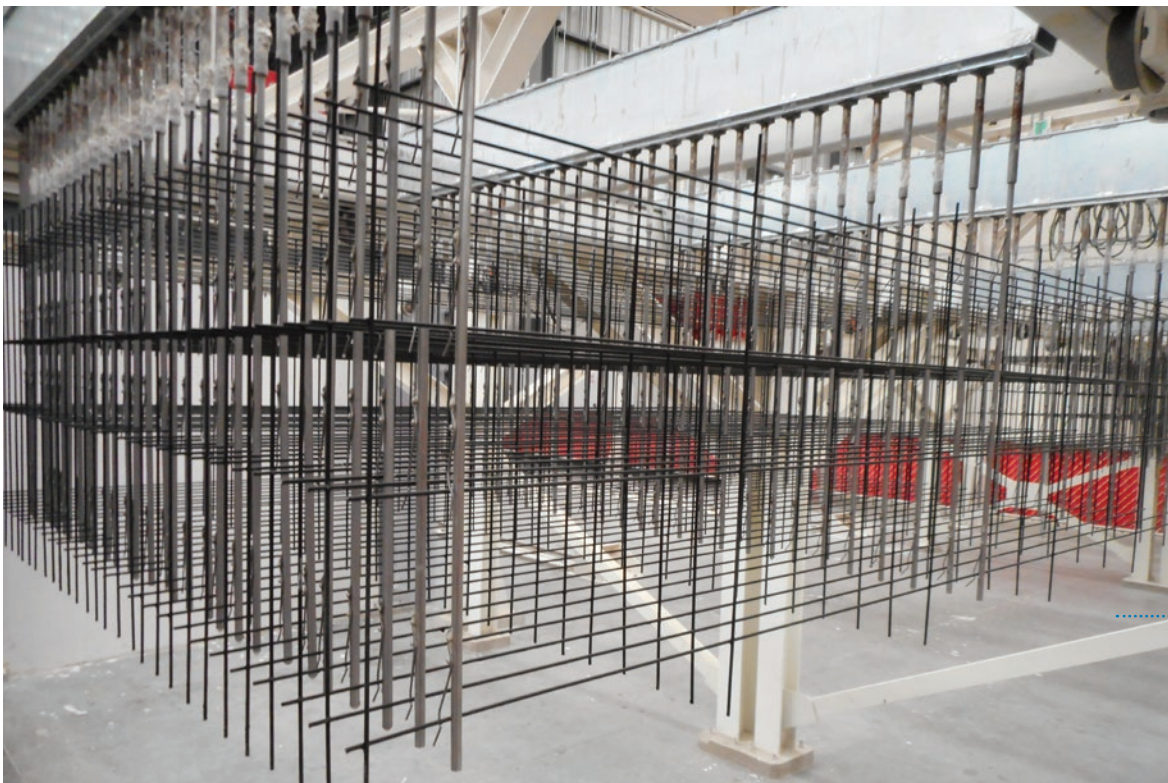
Fig. 3: A close-up view of the reinforcement assembly area prepared for thin panels.
