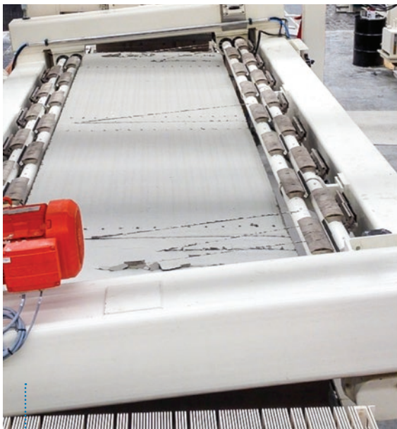
Fig. 4: Cutting panels with rest blocks leads to the most common problem of dealing with by-product blocks that does not fit market dimensions and densities.
