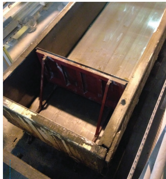
Fig. 5: Using damming walls inside the moulds for getting shorter cake lengths is one of the preferred options for plants with non-movable back doors.
