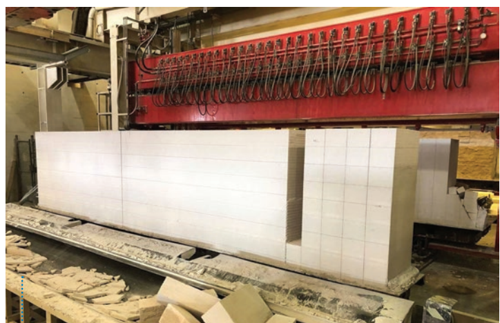
Fig. 3: The waste layer between the panels and blocks creates additional white waste that needs to be dealt with.
