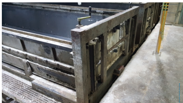
Fig. 7: Adjustment of the movable back doors are executed manually by releasing the outer frame on the movable back door and fixing it again at the desired length with clamping levers.
