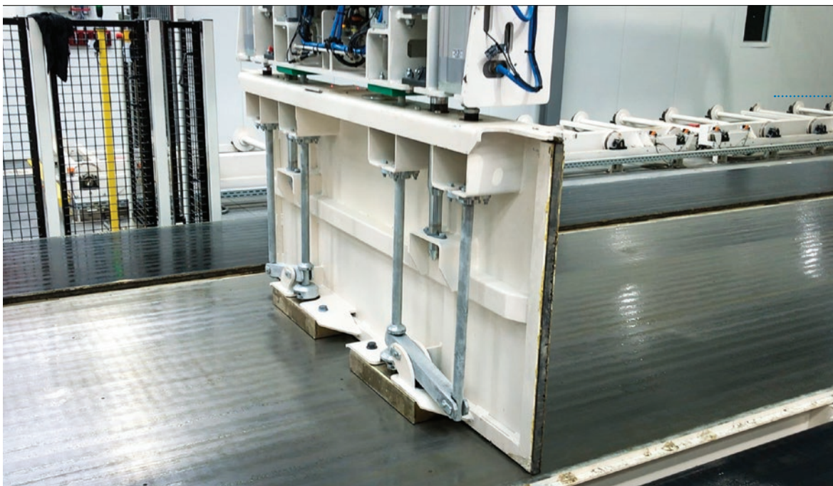
Fig. 9: The movable door is picked up by the door manipulator and placed on the desired position as per the configuration on the plant automation system.
