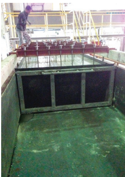
Fig. 6: Leakage of the mix is a commonly faced issue in moulds where all sides are fixed.
