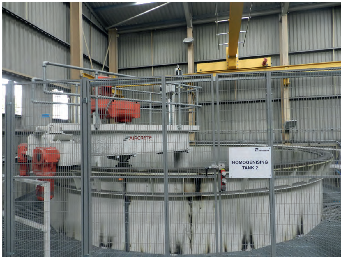
Fig. 9: Homogenising tanks make the slurry more homogenic by mixing up several batches of conditions ash in the large tank
