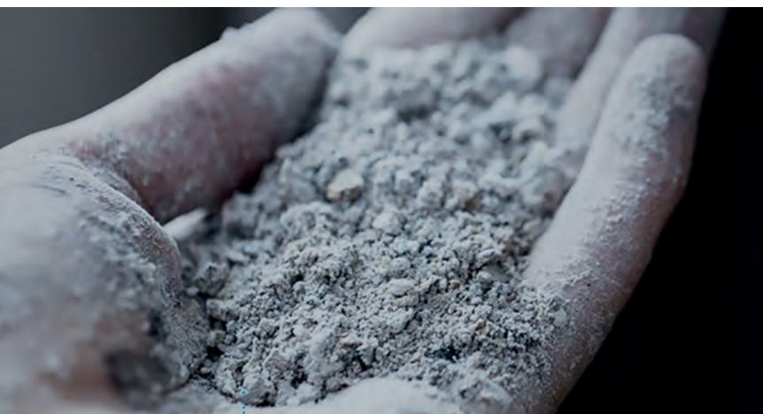
Fig. 1: Used in cement, AAC blocks, and a variety of other applications, fly ash, or Pulverised Fuel Ash (PFA), is an important material for the construction industry
