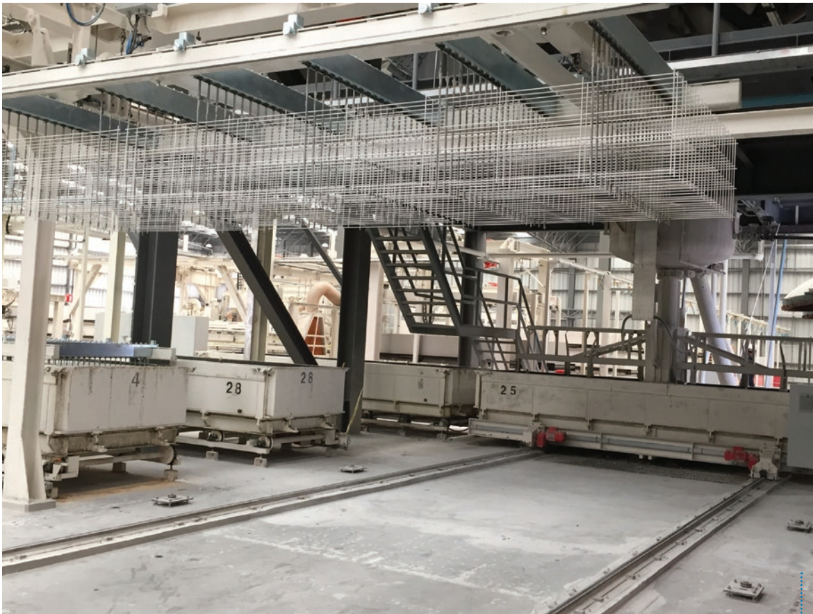
Fig. 5: A fully automatized reinforcement area brings in the desired flexibility level for product diversity and large volume requirements.
