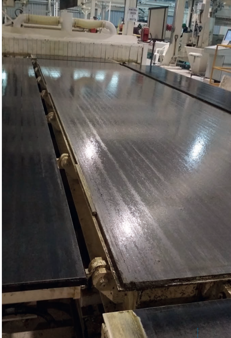
Fig. 4: The special design of the moulds makes it is very easy to clean and oil the mould using the automatic Aircrete mould brushing and oiling system.
