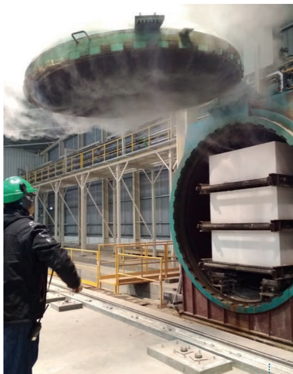
Fig. 7: No back-tilting or further transfer of the cake is required for autoclaving
