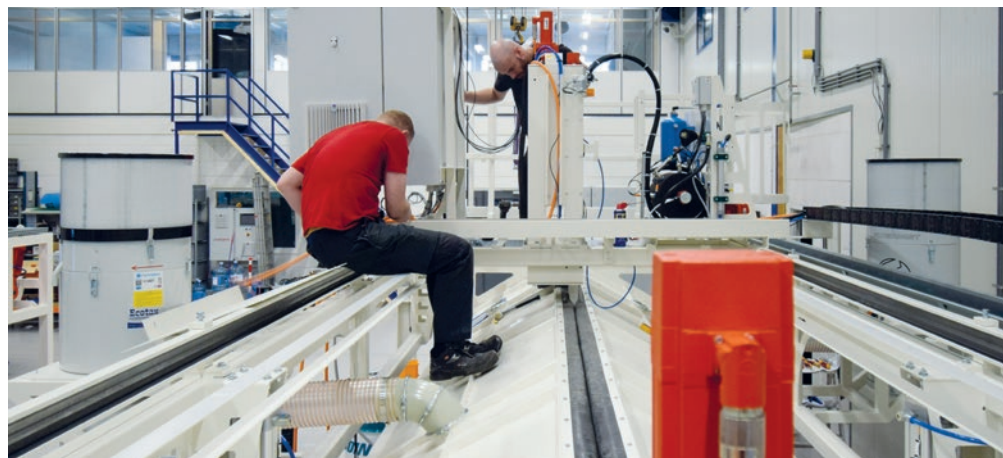
Fig. 6: Aircrete Europe engineers assembling the mould oiling system during workshop installation and testing.
