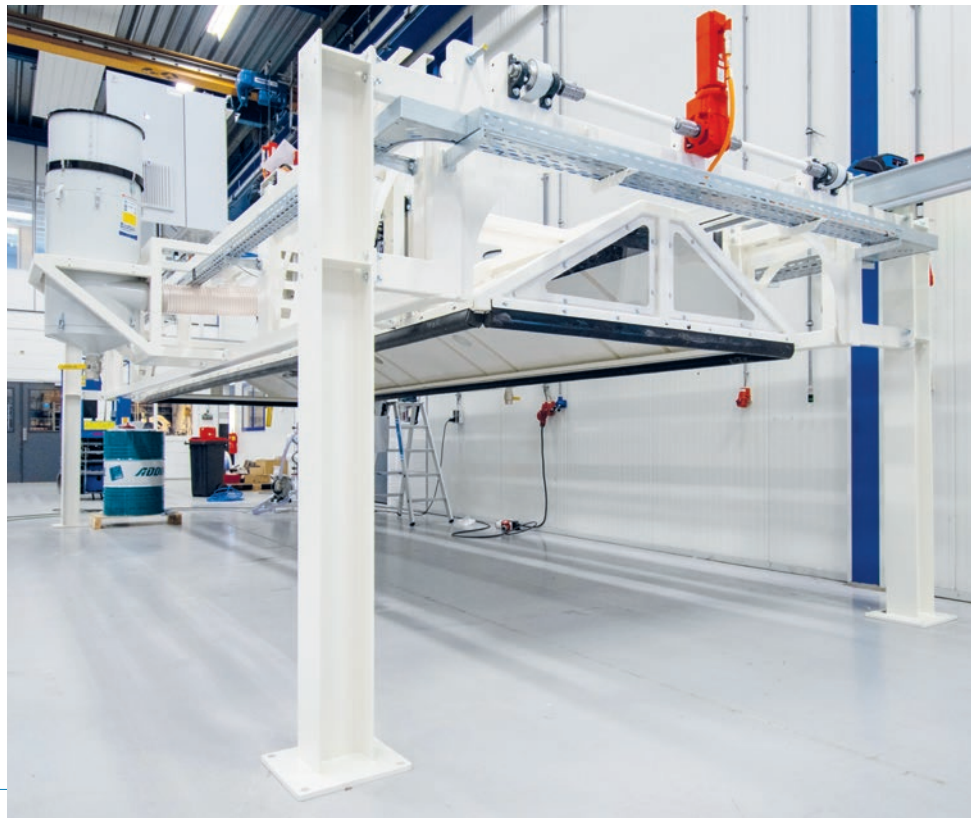
Fig. 1: Closed Mould Oiling Machine assembled at the Aircrete Europe workshop prior to installation in an AAC production line.
