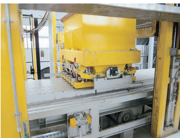
Concrete pouring unit filling U-blocks with reinforcement concrete under controlled conditions
