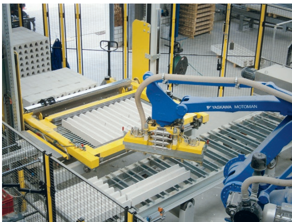
Robotic setting system placing U-blocks on circulating pallets for lintel production
