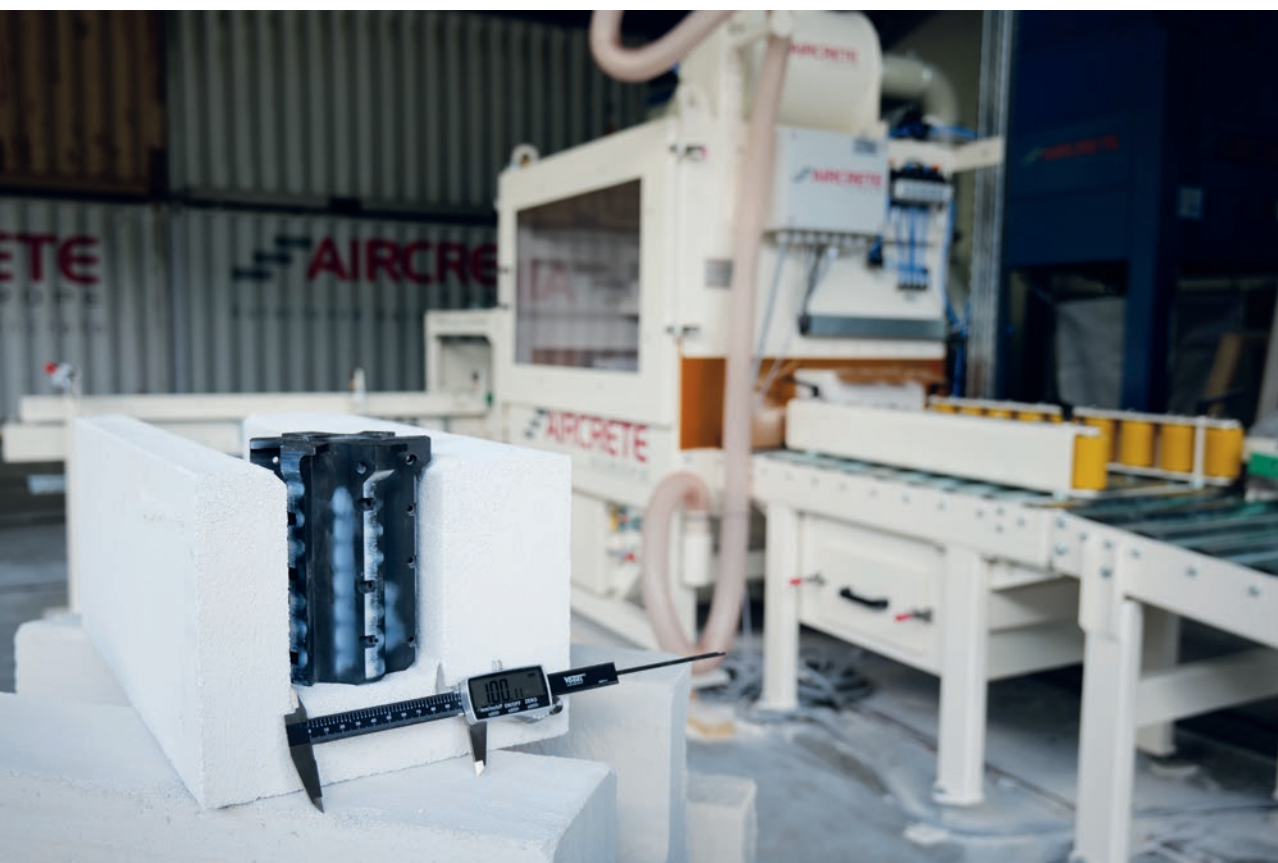
Finished AAC U-blocks discharged from the milling line
