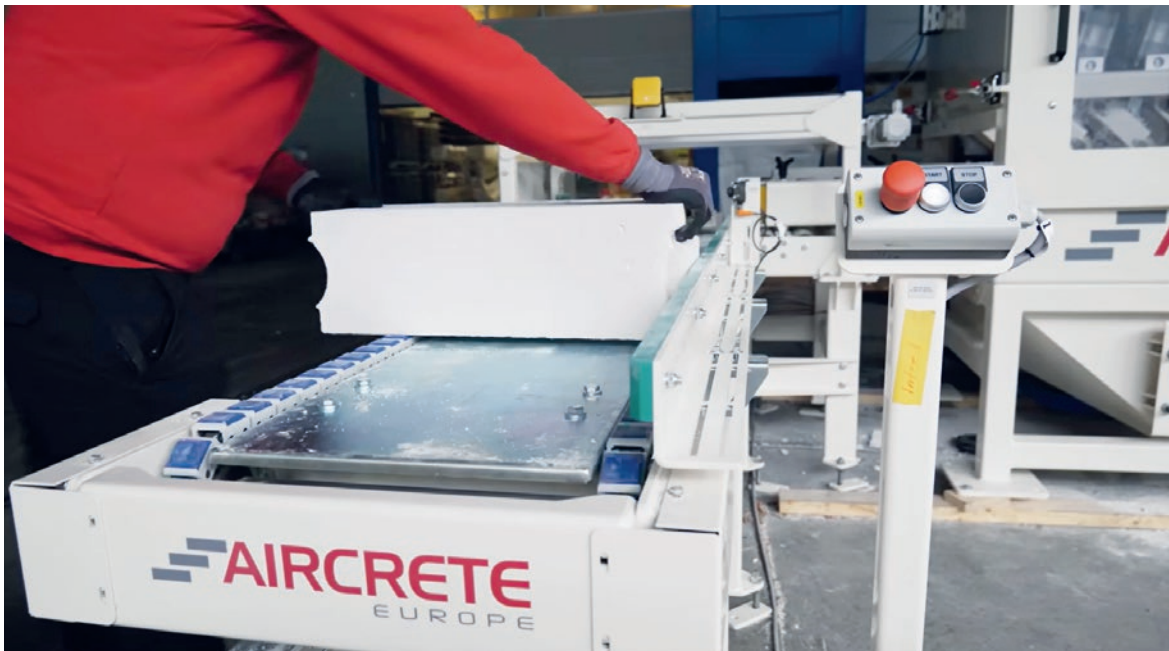
Operator view of the Aircrete U-block machine
