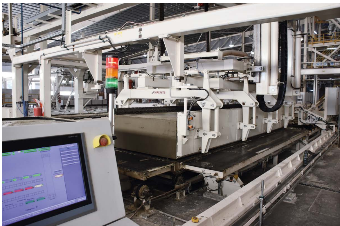
Fig. 7: Grabbing manipulator taking the cake from the open mould to move it onto the cutting line.
