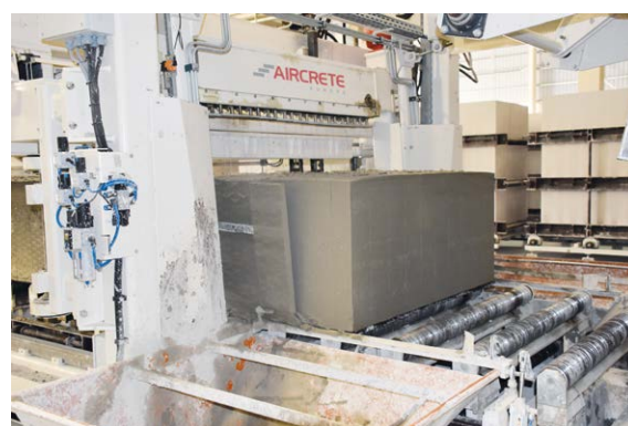
Fig. 8: Cross-cut cake going through the High-Speed Cutting Frame (HSCF).
