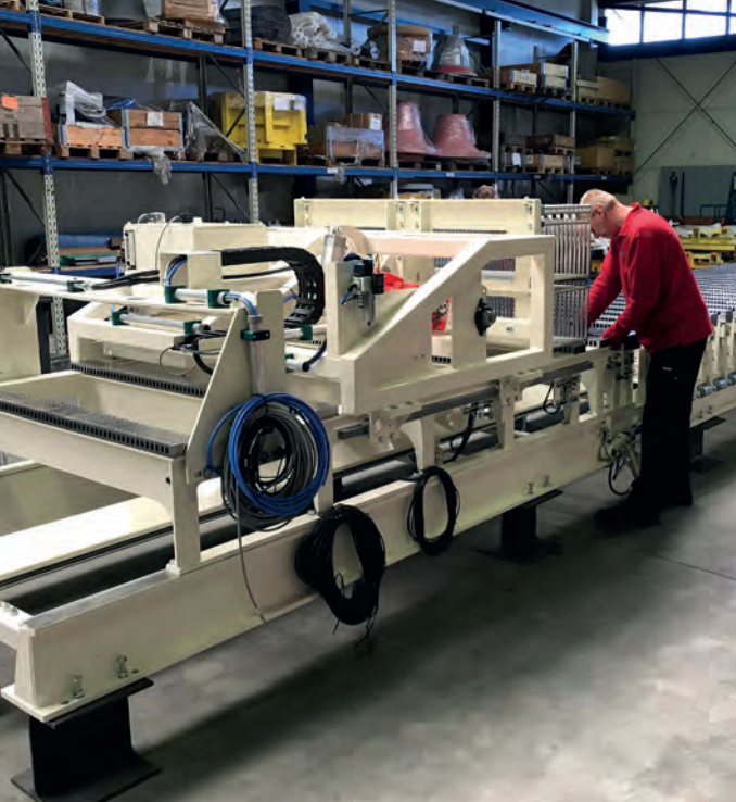
Fig. 7: New lamella table and pusher during testing in Aircrete workshop before departure to Celco, Romania
