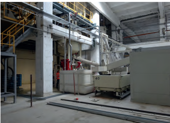
Fig. 1: Modern Aircrete design mixer discharging the mix into the mould
