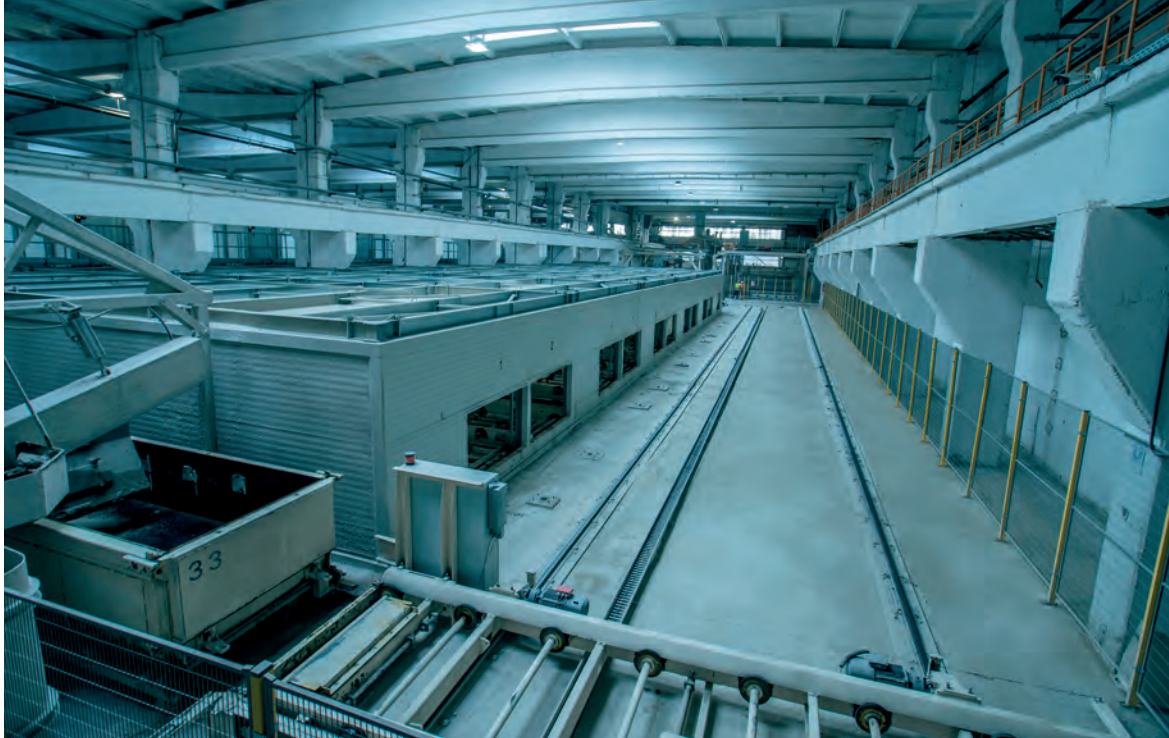
Fig. 5: Aircrete's mould rising area and moulding traverser car at Holcim, Romania
