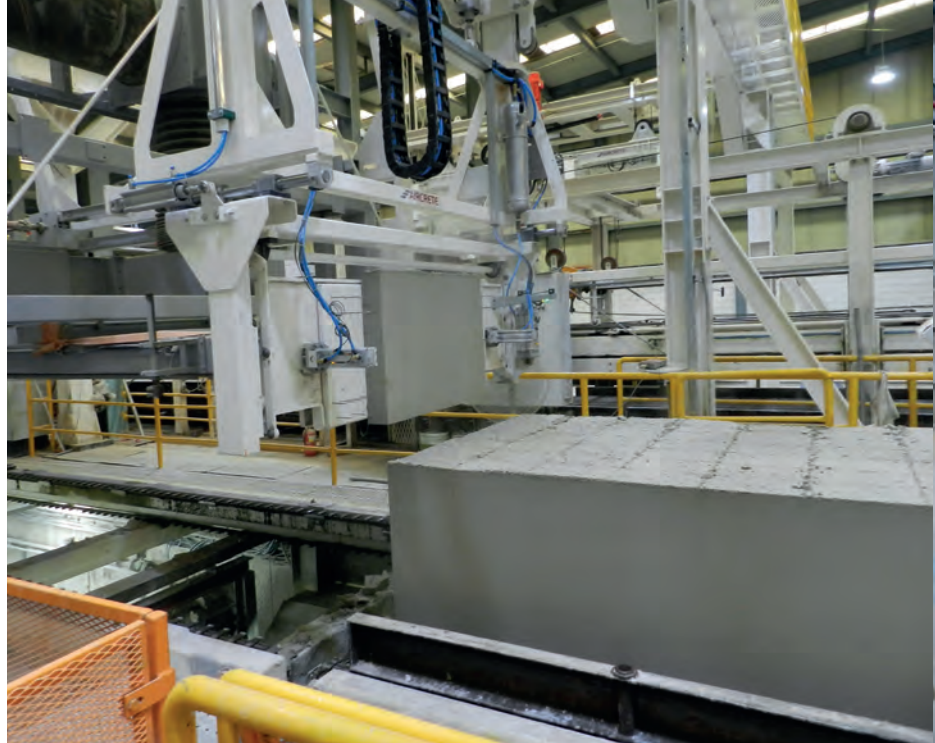
Fig. 9: Automatic end crust removal via nail plates at SYC, Korea
