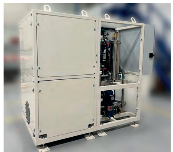
Fig. 2: Automatic high-pressure mixer cleaning system (pre-assembled)
