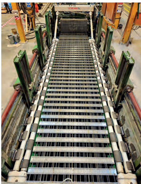
Fig. 6: Cross cutter with double-oscillating shafts with pneumatic tensioning at Q-Con, Thailand
