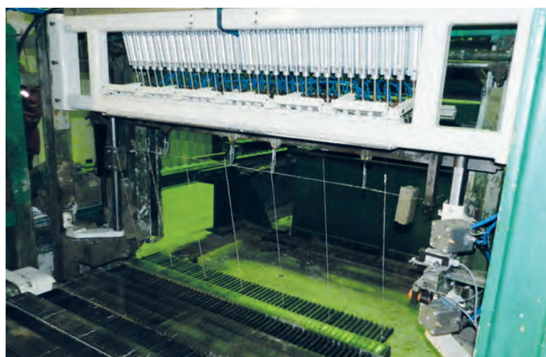
Fig. 8: Pneumatic vertical wires tensioning system in an old Hebel plant
