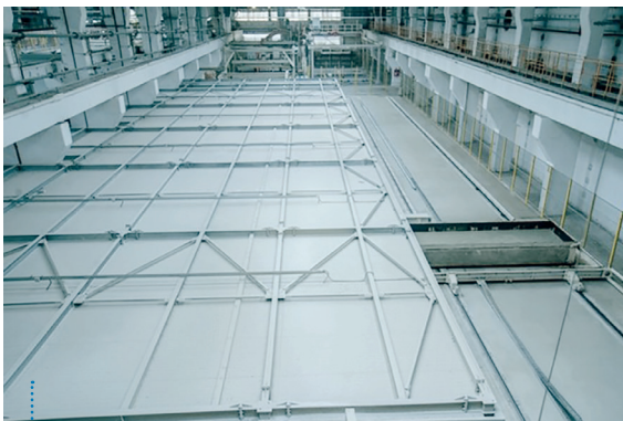
Fig. 3: A covered rising area, fully-equipped with a flexible roller track system, in one of Aircrete’s latest upgrade projects in an old Hebel plant in Romania.
