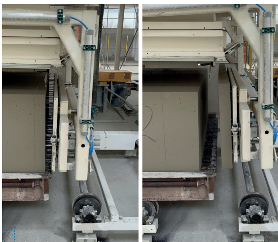
Fig. 9: Automatic removal of front and end crust to ensure an effective and safe removal of product.
