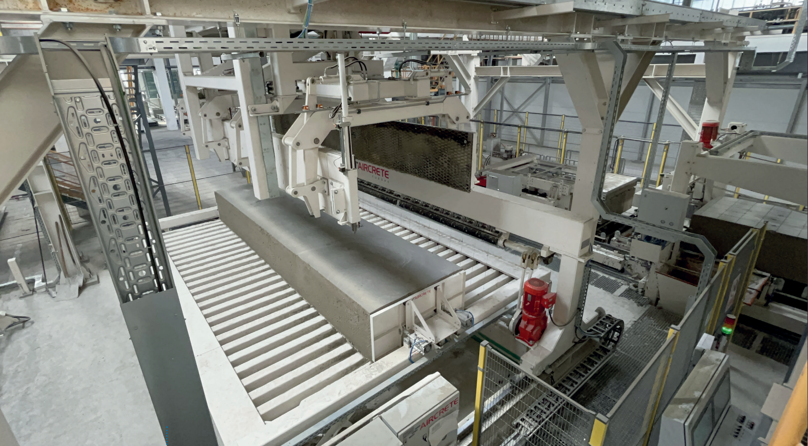
Fig. 7: A separate cross cutter ensures shorter cycle times and an even higher cutting accuracy.
