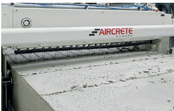
Fig. 8: The Aircrete High-Speed Cutting Frame creates a very good product surface on both blocks and panels.
