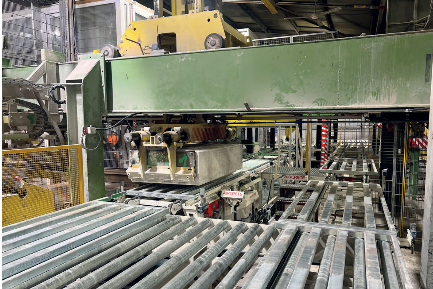
Fig. 1: Infeed grabbing manipulator putting a fresh half cake onto the packing line
