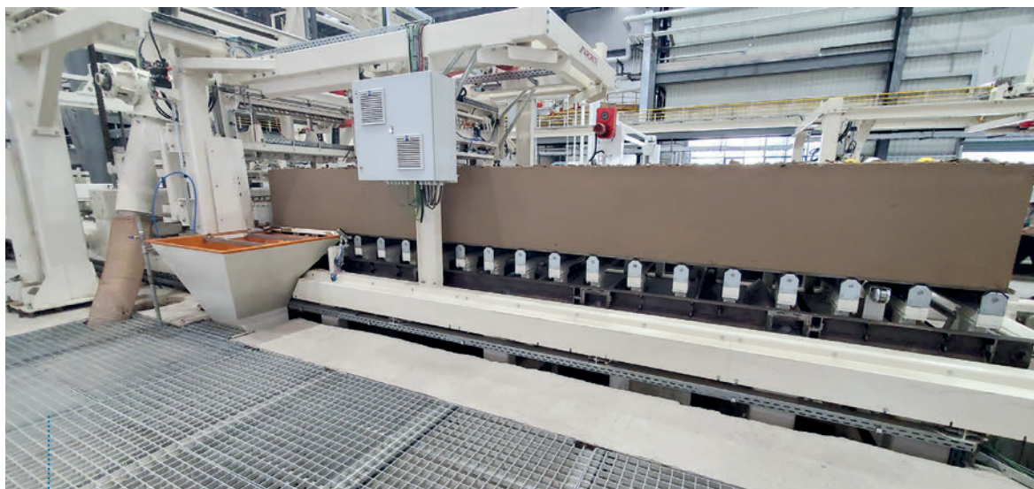
Fig. 7: In all Aircrete plants, the cake remains horizontal from casting, rising, cutting till unloading, and no separating nor green cake tilting machines are needed.
