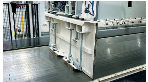
Fig. 6: The Aircrete Movable Mould Door in action: an automated door manipulator picks the movable door out of the door carrier and places it on the desired position.
