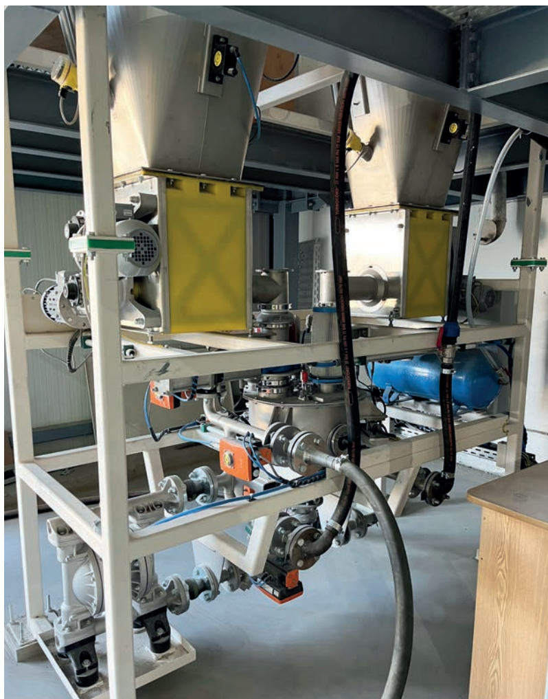
Fig. 4: The new Generation Aircrete Aluminium Dosing System
