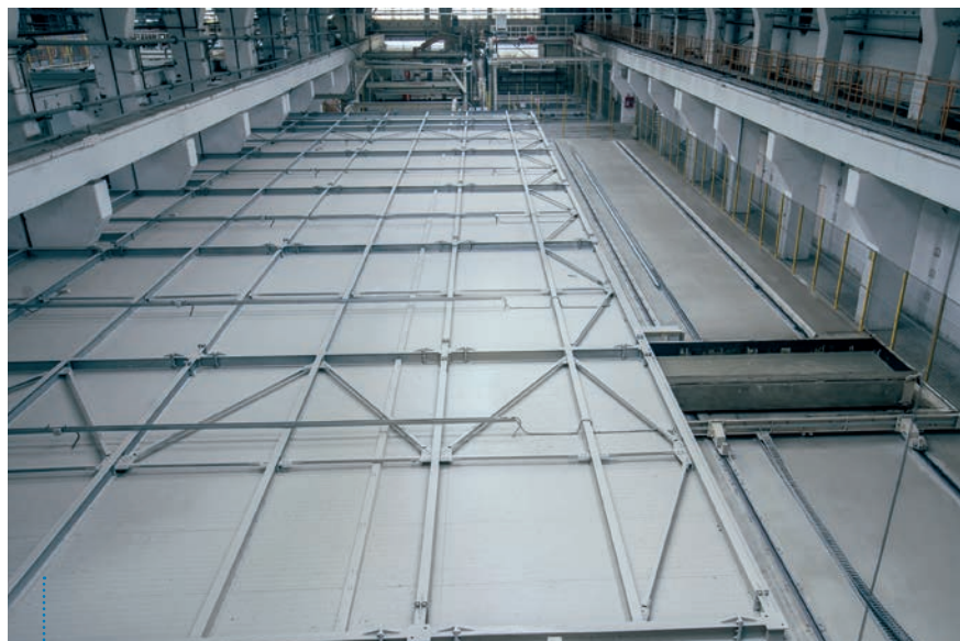
Fig. 3: The new rising area has been covered and fully-equipped with a flexible roller track system.
