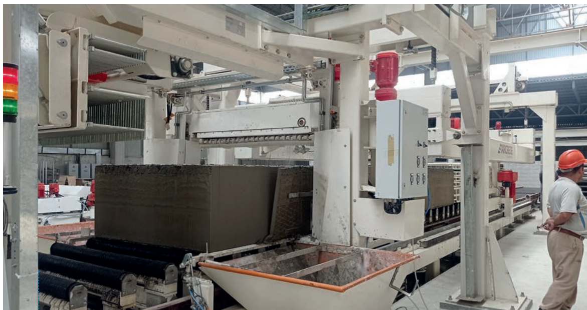
Fig. 2: The heart of an AAC factory with the unique Aircrete flat-cake cutting line
