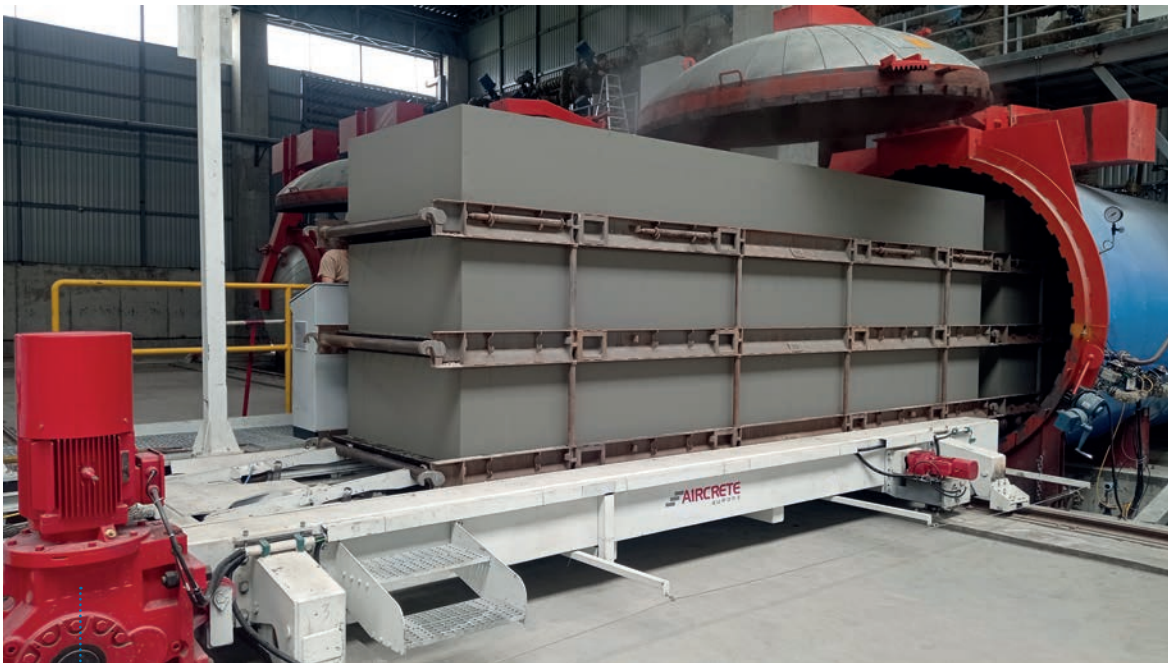
Fig. 5: Autoclave loading and unloading with the traverser car.
