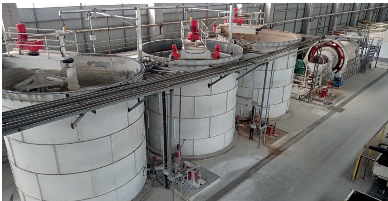
Fig. 3: The raw materials preparation area with 3 (150 m 3 ) slurry tanks and a 25 ton/hour ball mill.
