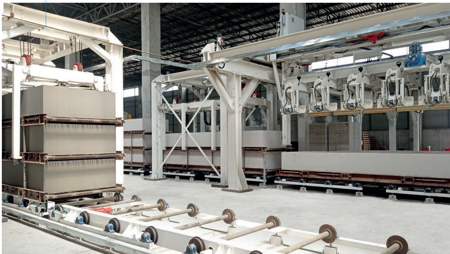
Fig. 4: Stacking of green cakes and de-stacking of white cakes on the background. Examples of equipment produced at Aircrete's manufacturing facility in China.
