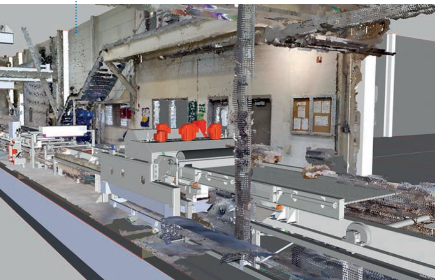
Fig. 10: Utilizing point-cloud technology allowed for smooth projection of new equipment in the existing facility (above – implemented, below – during design phase).
