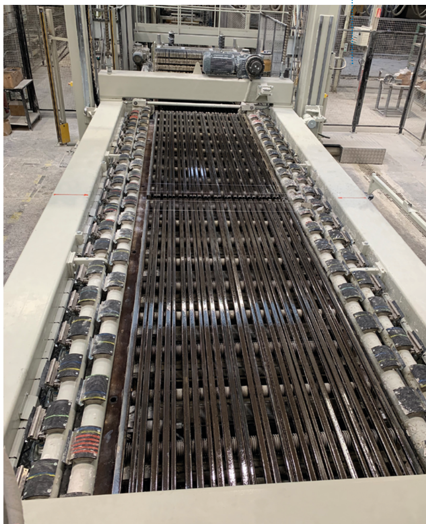
Fig. 2: The wires of the Aircrete Cross Cutter can be positioned on any position from 0 to 6 meters, with increments as short as 5mm.
