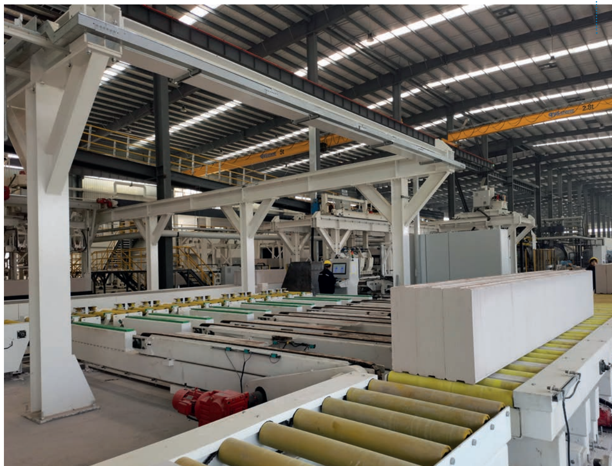
Fig. 9: In the unloading area, a crane takes the complete white cake and transfers them one-by-one from the frame onto a dedicated packing line depending on the type of product.
