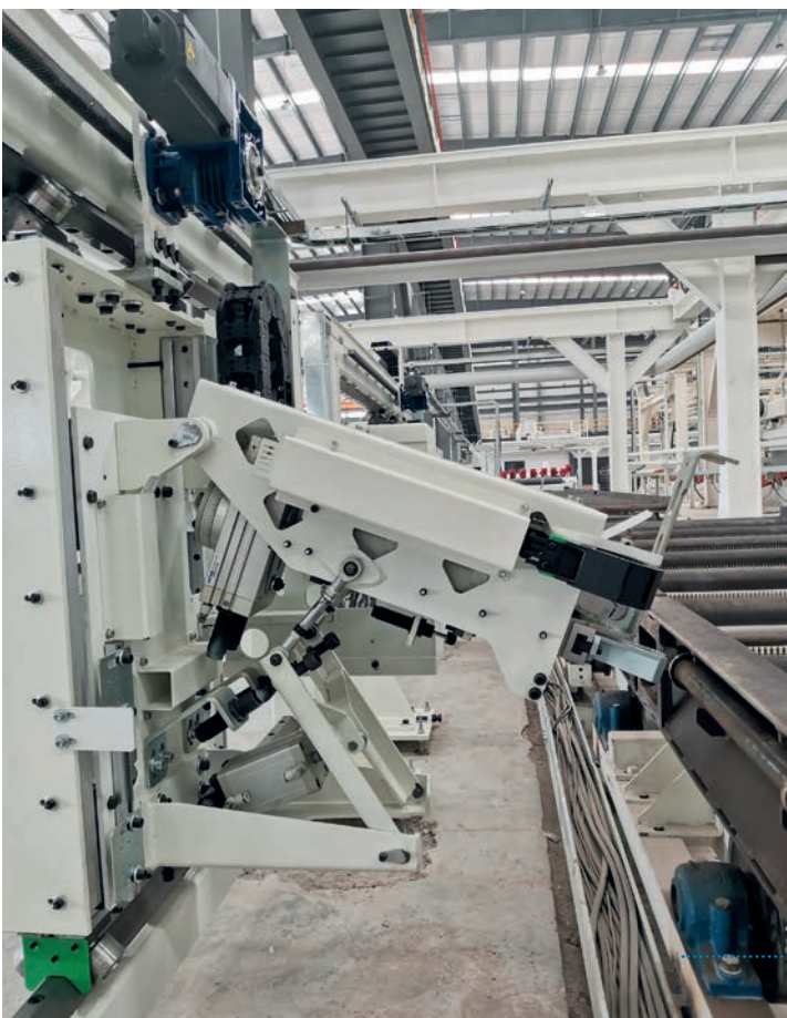
Fig. 8: The stacking pin manipulators insert pins automatically on the curing frames.
