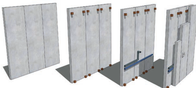
Fig. 11: Developed by Yuanzhu, the double-layer sandwich panel system is a ready wall solution that consists of two thin AAC panels with a gap in between.
