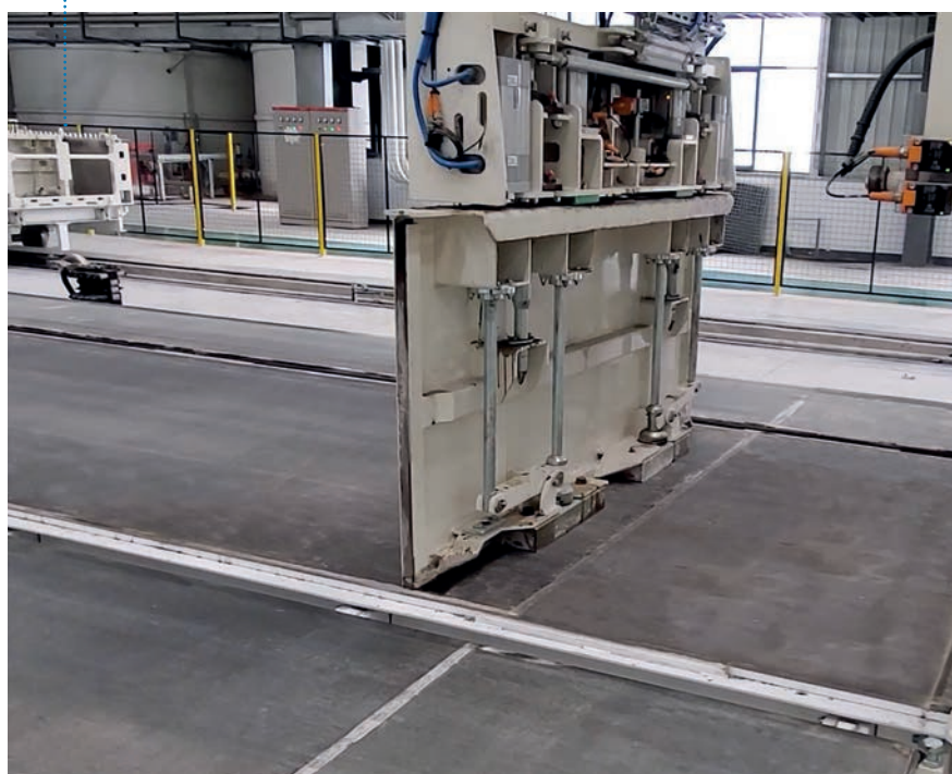
Fig. 6: The fully automatic adjustable mould doors allow to automatically adjust the mould length just before casting without the need of using separate damming walls.
