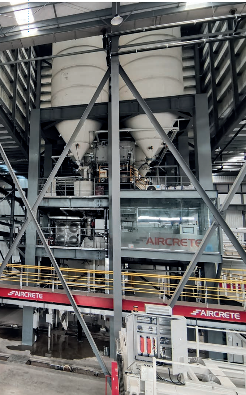
Fig. 4: Raw materials preparation, customized mixing ratios, dosing and mixing equipment are brought together in this project again as in all Aircrete plants, which is the prerequisite of high-quality AAC products.
