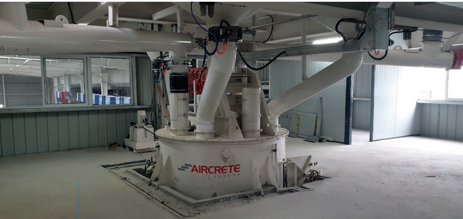
Fig. 5: The Aircrete low-speed mixer with multi paddles provides a homogeneous distribution of raw materials in the mix
