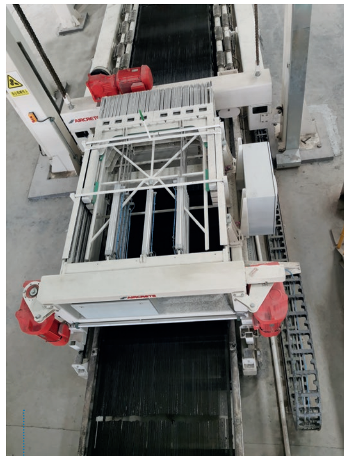
Fig. 10: A top view of the pusher and the cross-cutter of the Aircrete Cutting Line on site
