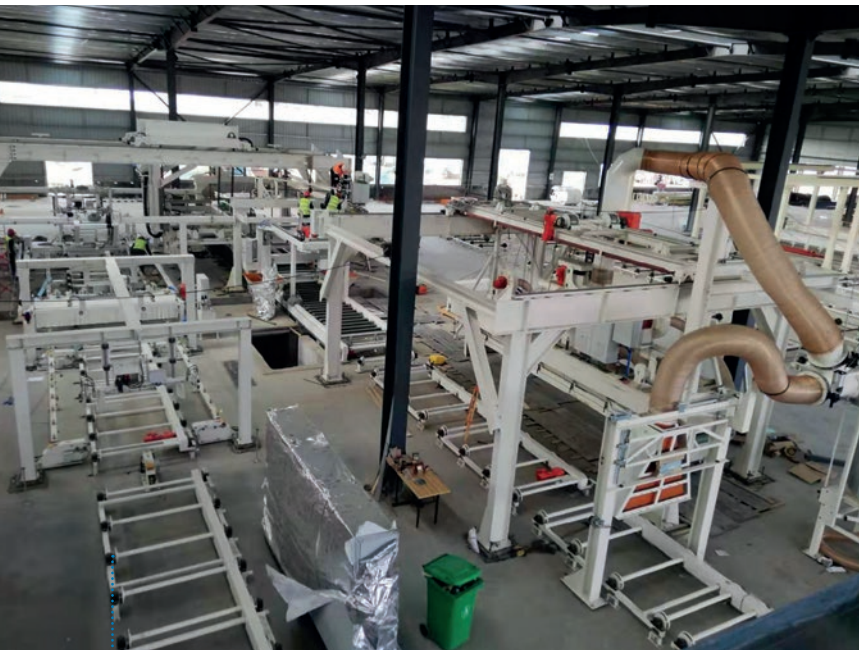
Fig. 9: In all Aircrete plants, the equipment foundations requirement is minimized to only the ball mill, mixing tower and cutting line
